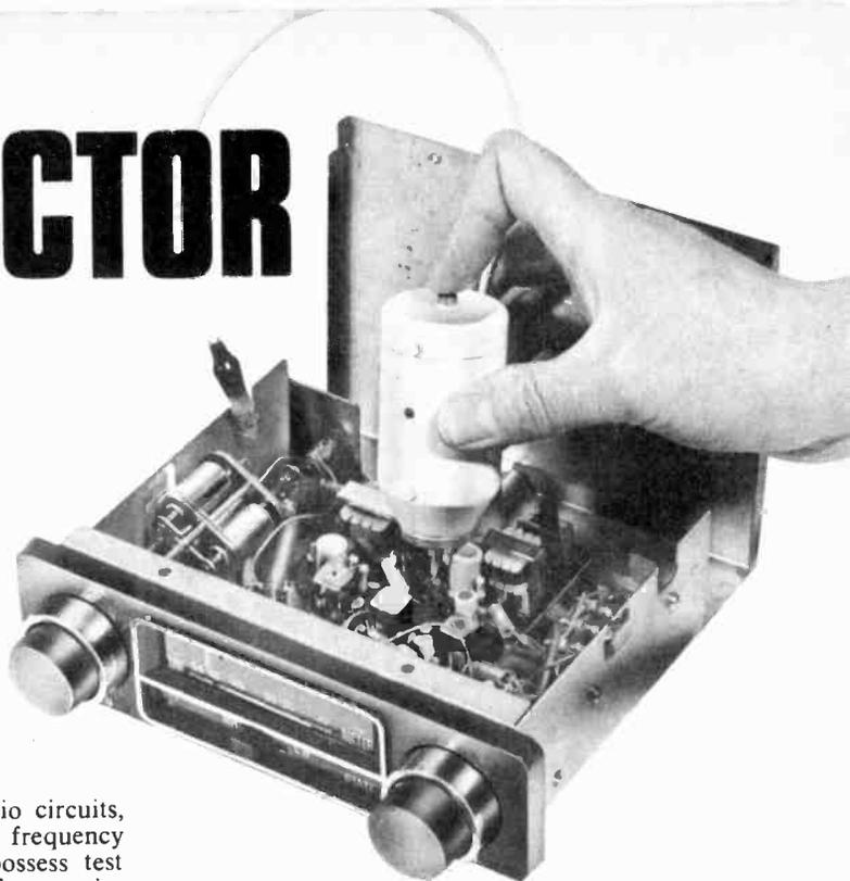
It is often necessary, particularly in radio circuits, to check for the presence of high frequency oscillations but most amateurs do not possess test equipment capable of responding to frequencies greater than a few megahertz. The probe described here will respond to frequencies between 200Hz and 30MHz, allowing use in general a.c. signal tracing. Any a.c. of a few millivolts or more will light a small light emitting diode (l.e.d.). The whole instrument can be held in one hand.
