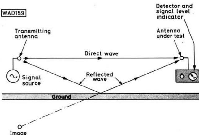
**Fig. 10.1: Direct wave versus ground reflected wave from the signal source antenna to the antenna under test**
