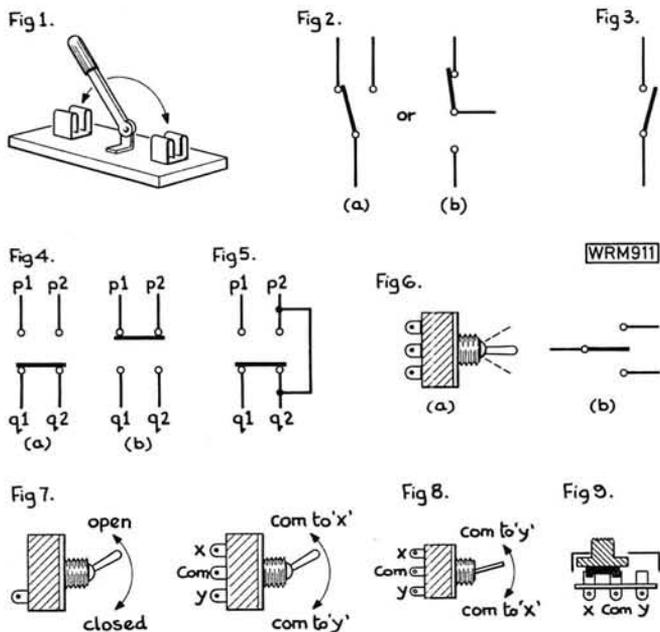
original position when you let go of it. In single-throw switches it's very often used to bias the action to the "OFF" position. In "centre-off" switches, biasing can be applied to return the dolly lever to the centre position. Sometimes both sides are biased to return to centre, in other switches one side is biased and the other is not.
