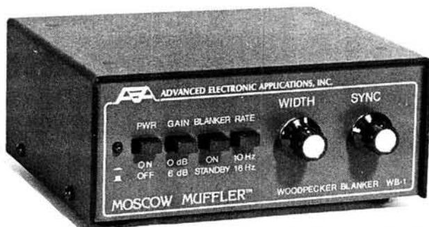
The AEA WB-1C is designed to be inserted into the 50Ω coaxial feeder between antenna and rig. It generates a steady stream of blanking pulses which control a gate in the antenna feed-line, isolating receiver from antenna when the pulse is present.
