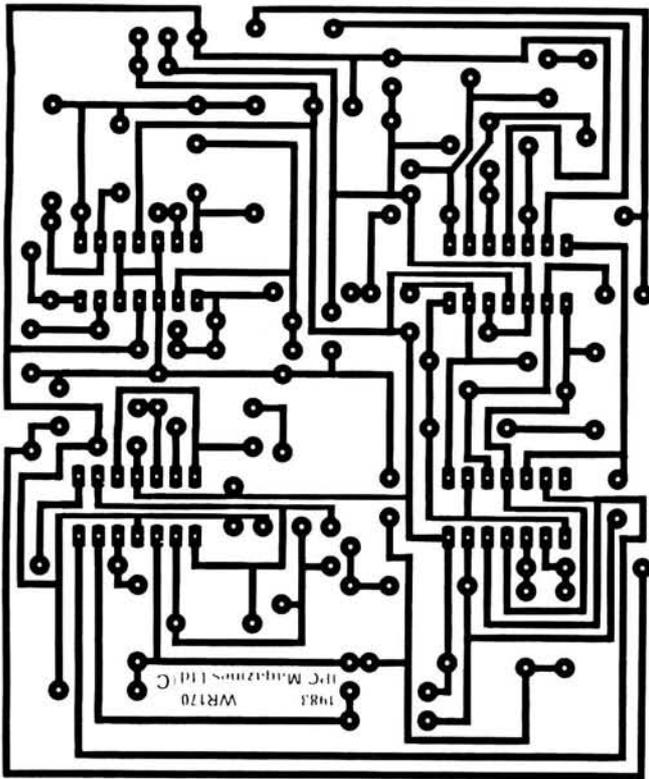
**Fig. 4: Component placement and p.c.b. track pattern of the d.r.i. shown full size. The waveform drawings shown opposite relate to the indicated points on the circuit diagram, Fig. 3**
