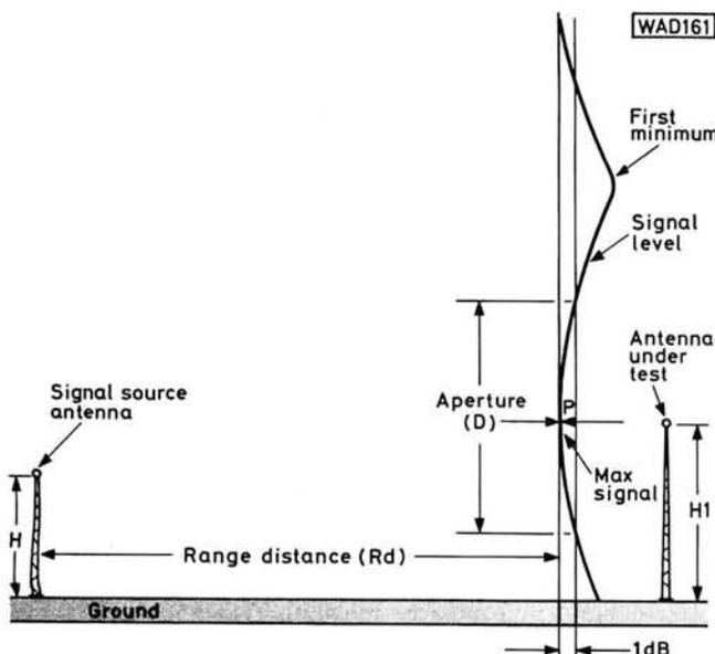
**Fig. 10.3: A plot of the signal level over the first maximum and showing the ultimate position (P) of the antenna under test**
