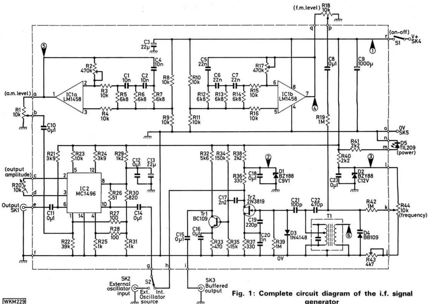
Fig. 1: Complete circuit diagram of the i.f. signal generator
