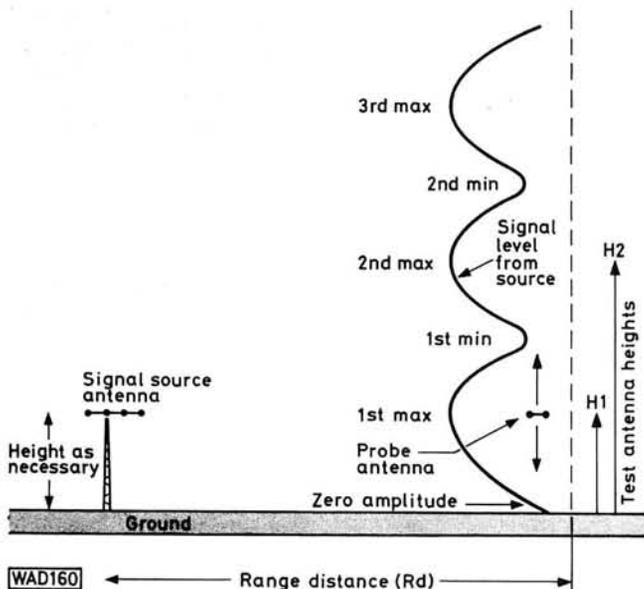
**Fig. 10.2: Profile of the signal level at the test site from the signal source**
