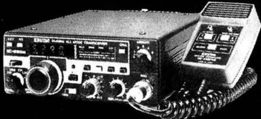
The recently introduced IC-290H has proved so popular that we have decided to concentrate on this (25W) model 2m multimode. With its bright green display, 5 memories, scan facilities on either memories or the whole band, tone-call button on the microphone and instant listen input for repeaters, this little box really is a beauty.
