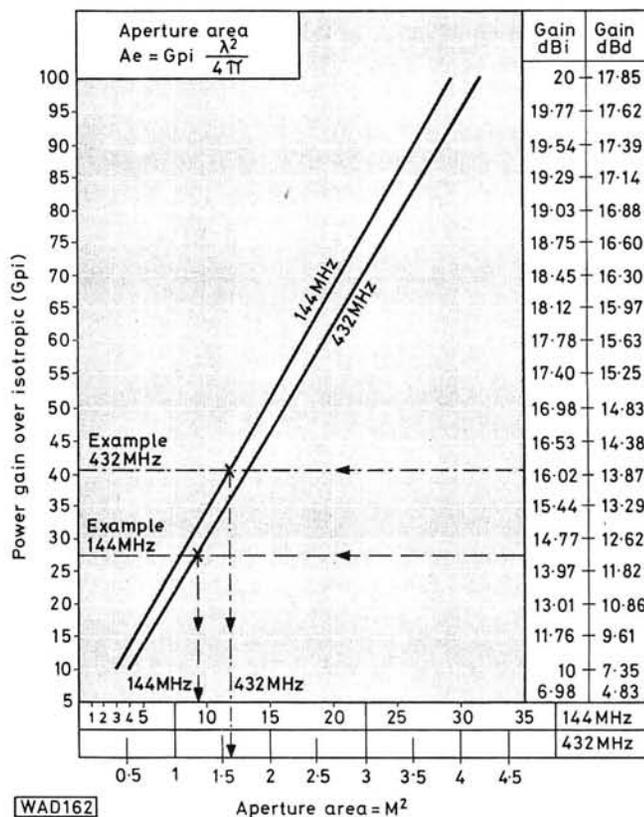
**Fig. 10.4: The aperture areas for 144MHz and 432MHz antennas with the gain factors in dBd or dBi (right hand columns) and relative power gain over isotropic in the left hand (Y) column. Examples are shown with dotted lines**
