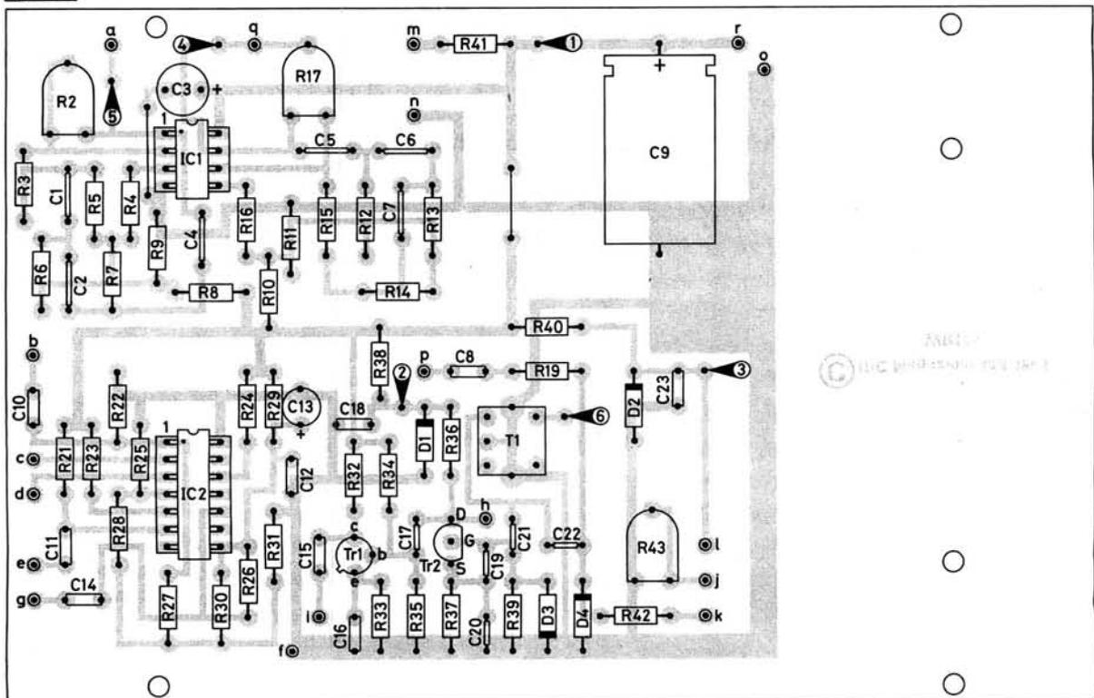
Fig. 2: The track pattern and component placement details of the i.f. signal generator
