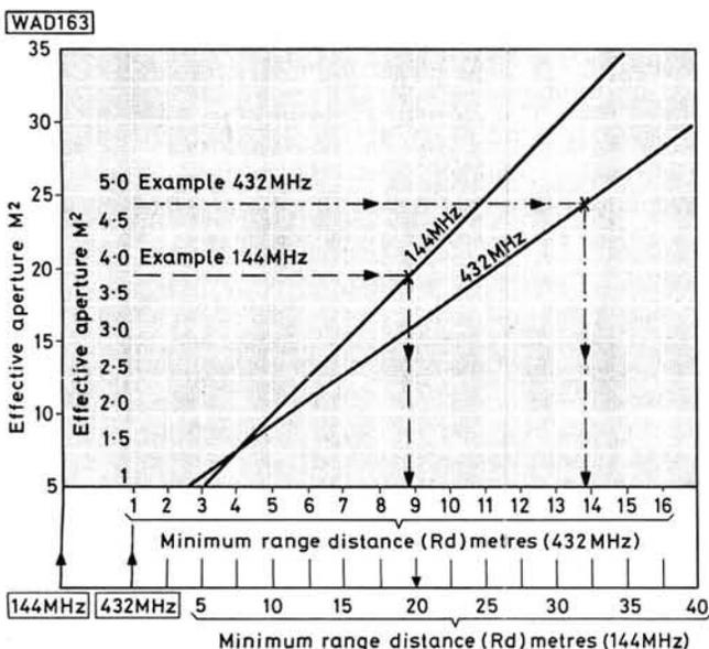
Fig. 10.5: The graph shows the minimum range requirement ( $Rd_{min}$ ) for various effective apertures for both 144MHz and 432MHz antennas
