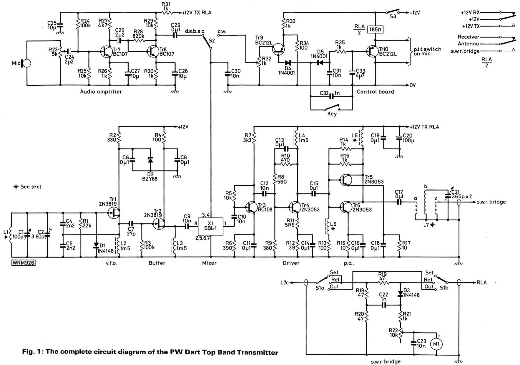
Fig. 1: The complete circuit diagram of the PW Dart Top Band Transmitter
