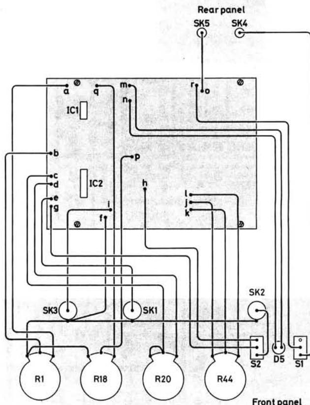
Fig. 3: Interconnecting wiring diagram between the p.c.b. and the panel mounted components
