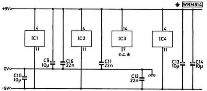
**Fig. 5: Supply rail and de-coupling arrangements. Note that pin 7 of IC3 is not connected**
