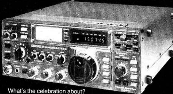
What's the celebration about? The IC-745...a new all band HF transceiver with SSB, AM, CW, RTTY and an FM option... plus, a 100KHz - 30MHz general coverage receiver. And...the IC-745 has a combination of features found on no other transceiver at such an incredibly low price. See the IC-745 at our shop and showroom at Herne Bay or contact your local authorised ICOM dealer for more information.
