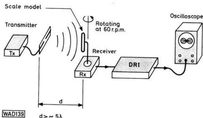
**Fig. 1: The basic test set-up required to evaluate receiving transducers e.g. scale model antennas, directional microphones or photocells. The motor driving the model antenna rotates at the same rate as the d.r.i. scan. A full display will be provided on a high persistence or storage type oscilloscope**
