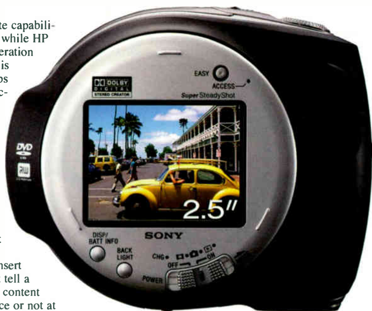
The Sony DCR-DVD7 DVD camcorder can be held like a digital camera: it has a 2.5in. screen touch-pad.
