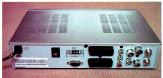
Photo 2: The rear panel, where the sockets and a mains on/off switch are mounted.
