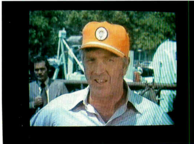
Photo 7: Some DVB-T channels are shown in 4:3 aspect ratio but not full-screen, with a black band all round.
