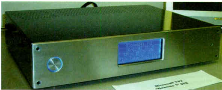
A prototype Microsoft IPTV (Internet Protocol TV) unit. IPTV enables TV programming to be distributed via the internet.
