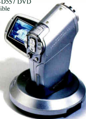
The Sanyo VPC-C4 camcorder uses MPEG-4 compression and offers 8-Megapixel resolution – by using interpolation to up-convert the signal from the unit's 4-Megapixel CCD image sensor.
