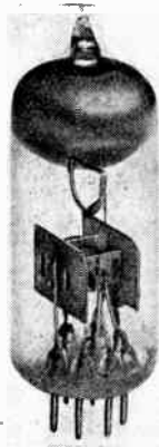
Fig. 3. Experimental parallel electrode triode (E1714) on pressed glass base.
