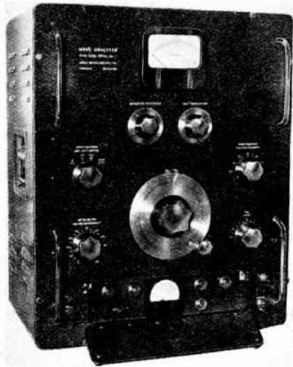
Dawe wave analyser for measuring component frequencies of a complex wave
