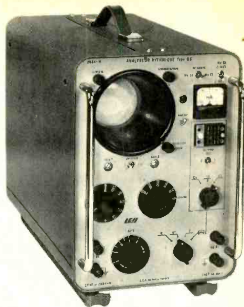
Instrument for measuring distortion on telegraph circuits, including a signal generator for signal speeds of 50-2400 bands (Laboratoire Electro-Acoustique of Paris).
