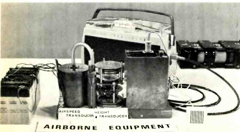
This photograph shows the complete airborne equipment comprising transducers, tape recorder and batteries.
