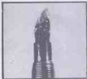
An ordinary Copper bit after 12,500 joints
