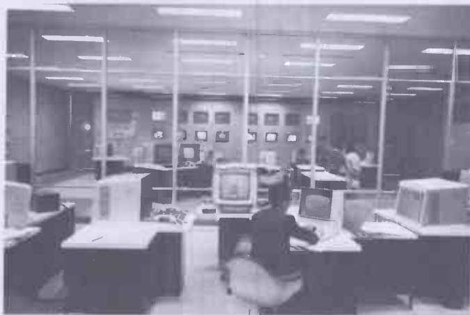
Tokyo control centre of the Japan Broadcasting Corporation's computer system 'TOPICS' which organizes and operates two television and three radio networks. The display unit in the middle gives managers access to all information on programmes in the course of production.
