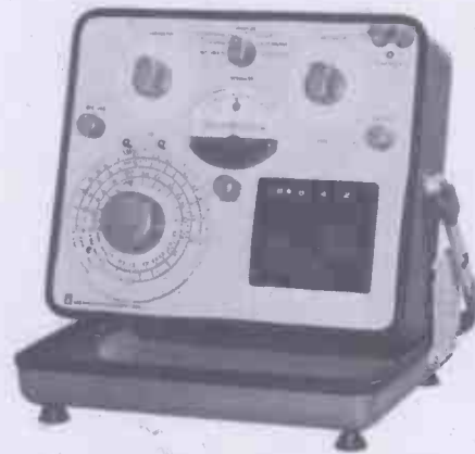
Fig.9. General Radio 1656 impedance bridge showing the digital CGRL controls.
