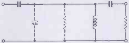
Fig. 2. Stray capacitance and conductance cause less h-f attenuation if the filter has no terminating resistance at the input end.
