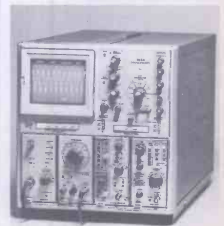
Fig. 7. Tektronix 7504 oscilloscope with the 7D13 digital multimeter and the 7D14 digital counter as well as a vertical amplifier and timebase.
