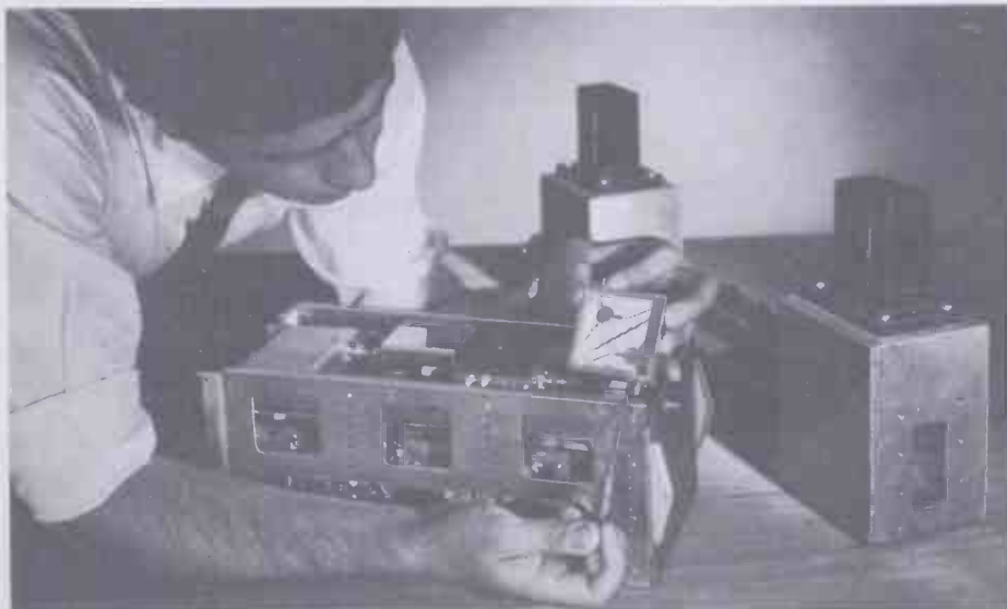
Prototype double converter for new Goonhilly aerial comparing Marconi microstrip package against conventional waveguide equivalent (right). Microstrip circuit includes two circulators linked by bandpass filter on an alumina substrate.
