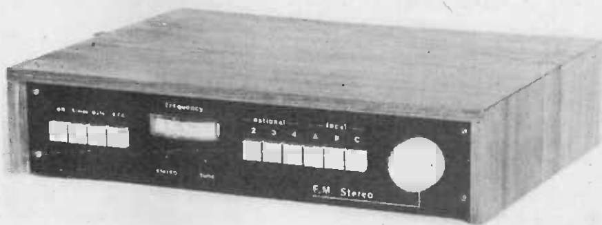
Features of this simple-to-operate stereo tuner include a muting circuit to prevent unwanted signals being heard (e.g. weak stations, signals affected by flutter, and mistuned stations), a single-lamp tuning indicator and a linear frequency meter.
