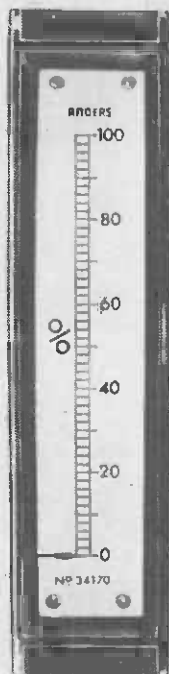
Profile 350 edgewise 4.3" scale. DC moving coil and AC moving coil rectified. Horizontal or vertical mounting.
