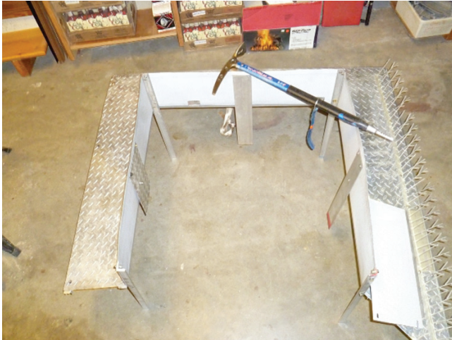
Figure 3. The nearly completed structure is constructed of aluminum siding, plastic spikes (right) and steel coils (not yet added) to prevent crows from landing on the lip of the Frank Wagner Elementary School chimney roost site in Monroe, WA. Photo by © Larry Schwitters.
