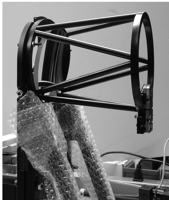
Fig. 11 Telescope frame held to the test fixture via kinematic mounts. The off-axis primary mirror is visible at the left end of the frame
