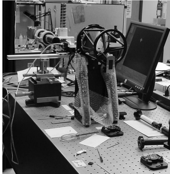
Fig. 12 Secondary mirror alignment phase with PSM behind the telescope, the image spot on the PSM computer monitor and kinematic locating bases for the posts (lying on their sides) and balls that define conjugate locations
