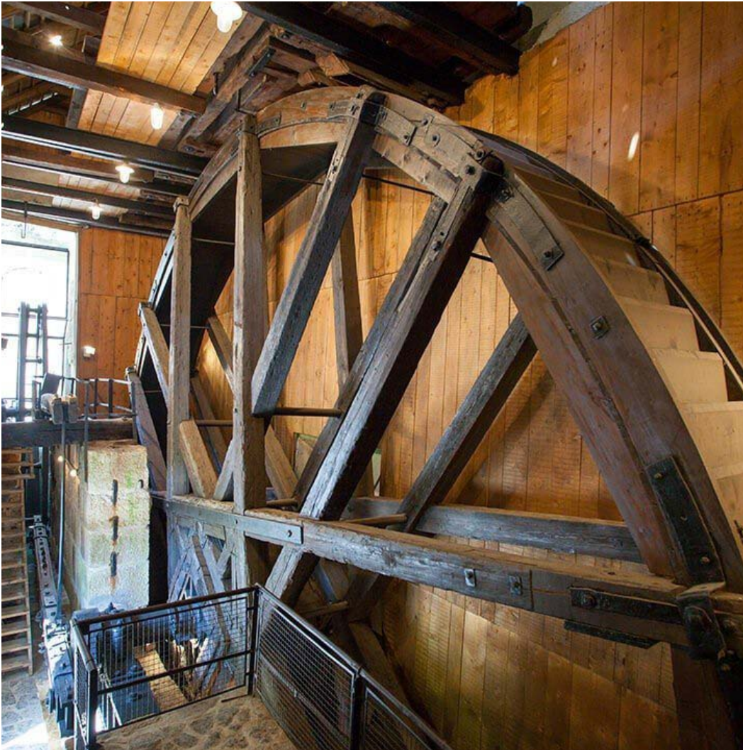
Kamšt, the water pumping wheel of the Idrija mine. (Idrija Municipal Museum)
