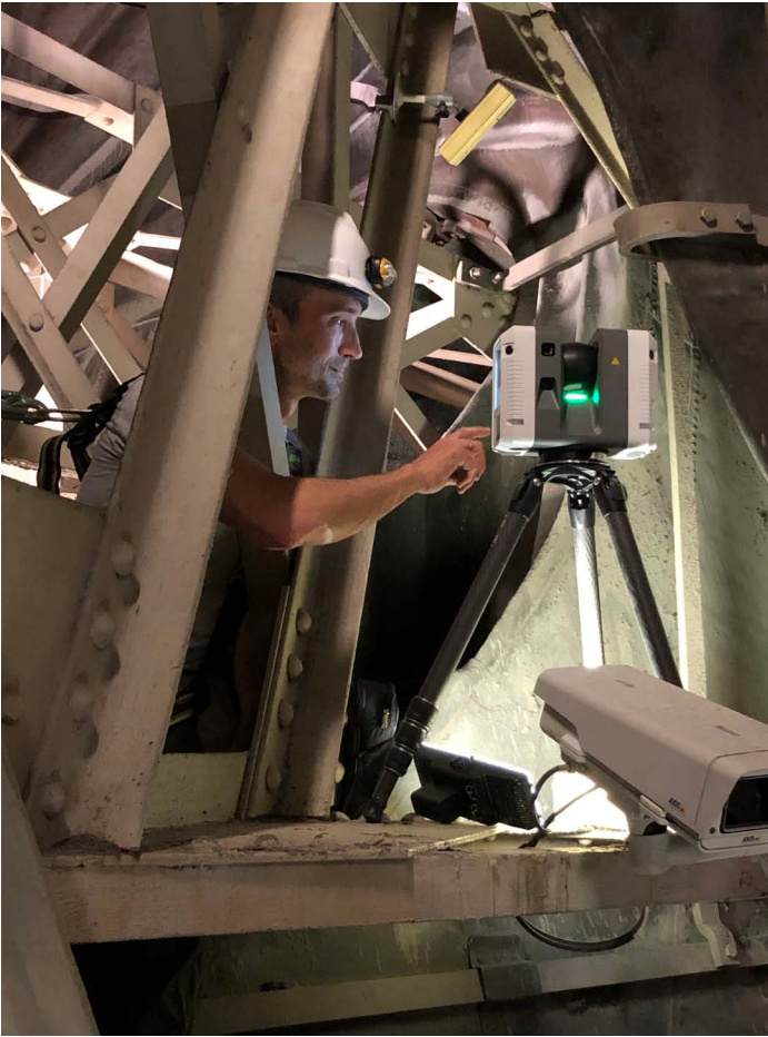
Architect Paul Davidson scanning the interior structural framework for a 2019 HAER survey of the Statue of Liberty.
