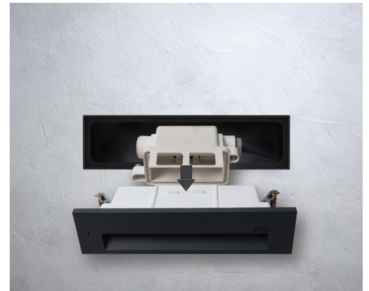
Step 1: Terminate the main cable(s) in the terminal box. Clip the terminal box on to the back of the luminaire.
