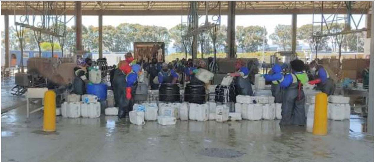
The facility has a dedicated area where night soil is delivered on a continuous basis, emptied, and treated, while empty containers are cleaned and recycled back for reuse. This facility provides work for casual workers.
