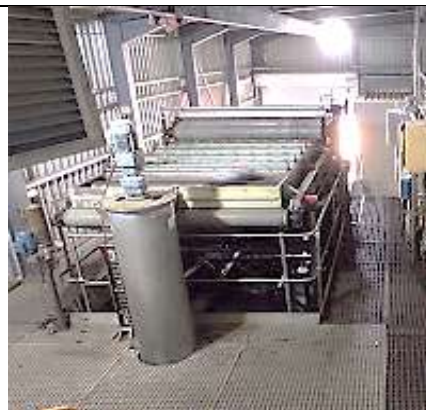
A well operated belt press system ensures a dry sludge which is taken away at regular intervals to the landfill site.
