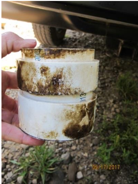
Figure 30. Cup used to hold juvenile mussels within silo. Cup is screened on both ends to allow flow through and splits apart to allow insert or removal of mussels.
