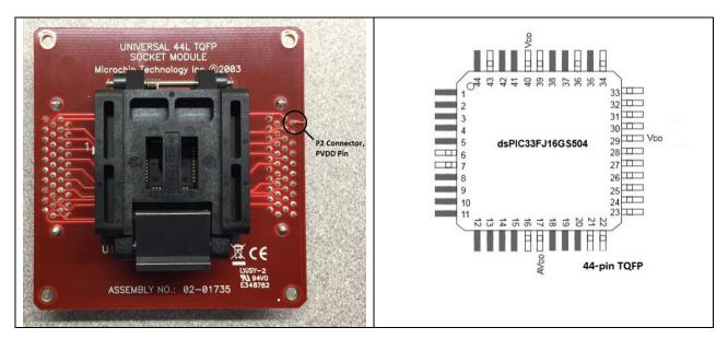
The goal is to provide the  $PV_{DD}$  high-current voltage source directly to the  $V_{DD}$  (pins 17, 29, and 40) of the TQFP device while removing the current  $V_{DD}$  connections.
