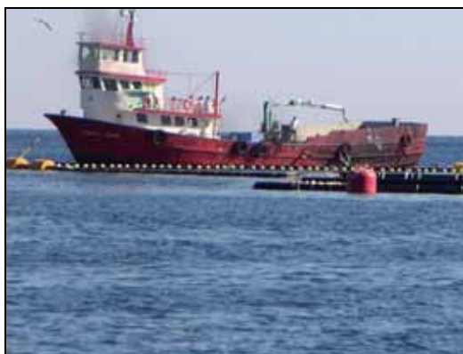
TS2: length 32m made of sheet iron. Feeding boat.
