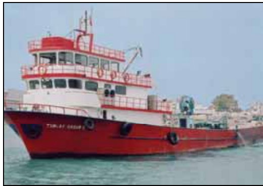
TS1: a ship with length 45m made of sheet iron. Berths 20 persons. Crane for 20tons, tank with 4 cooler systems and freezer. Also the generator and ice machine (providing ice from sea water)
