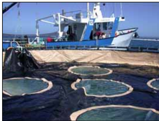
The mesocosm showing the only way in and the only way out (on the left). The clear circles are windows allowing researchers to see the fish and the fish to see daylight. The 16m SARDI vessel Breakwater Bay, from which most of the logistical work was carried out, is moored to the pontoon. Photo: Quinn Fitzgibbon.
