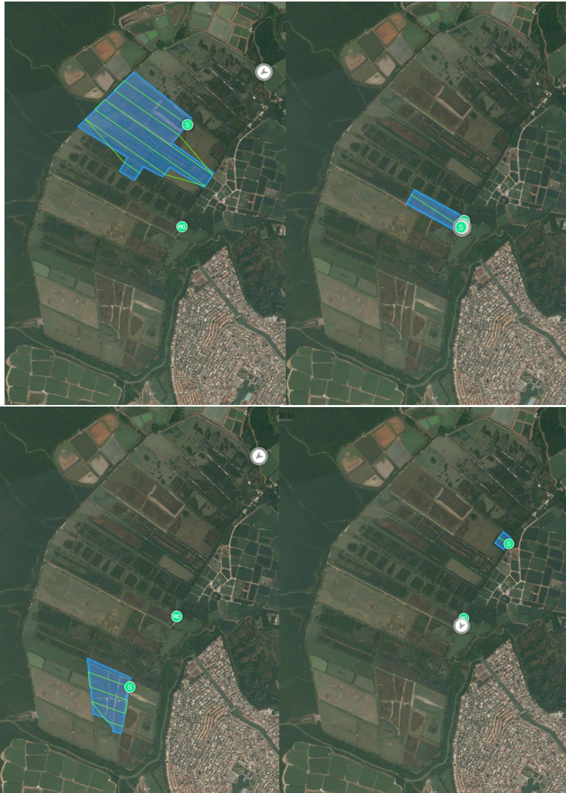
Figure EM05-2: Flight path for monitoring the health condition of specific reedbeds (areas to be covered are in blue and drone paths are in green)
