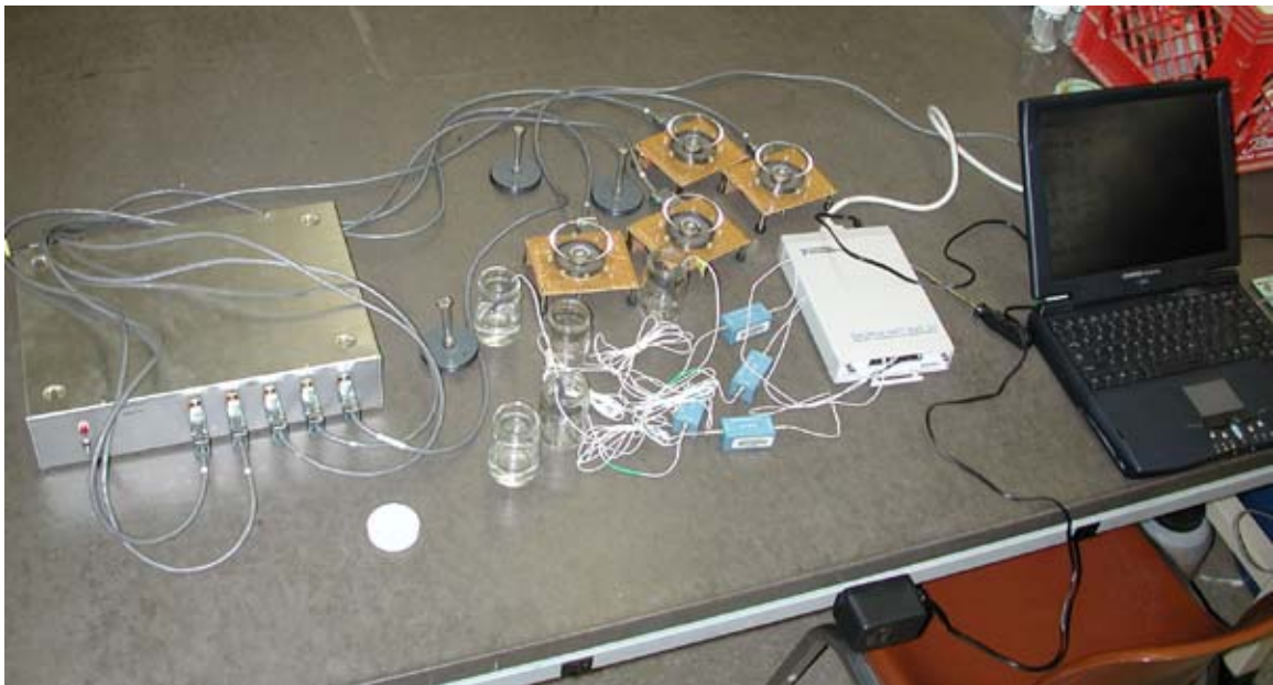
Figure A1-9. Another view of the apparatus. The custom made box to the left (described in the Quarter 2 report) converts the activity meter infrared detector signals (center, rear) to a voltage readable by the analog to digital board (just left of the laptop). Activity data and oxygen data feed into the analog to digital board, which then transfers converted data to the laptop.
