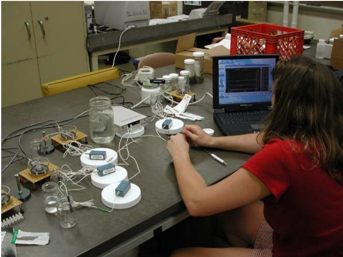
Figure A1-8. Attempting (unsuccessfully) to solve the problems with the oxygen probes. The white plastic circles were intended to isolate the oxygen adapters, which convert the signals from the oxygen microelectrodes (here in glass jars) to signals which can be processed by the analog to digital board. Activity chambers are in the background on left.
