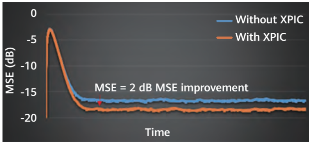
Figure 16 Polarization interference cancellation performance
