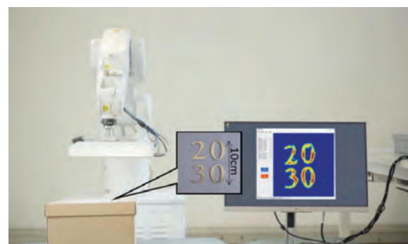
Huawei's ISAC-THz prototype achieves millimeter-level imaging resolution for objects in a closed box
