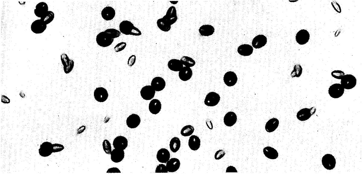
Figs. II-28 and 29. Fission Tracks. Photo above resulted from a Pacific Northwest Laboratory study of fission tracks and shows an irradiated sample of ordinary glass microscope slide coated with a thin layer of fissionable uranium. These tracks are actually trails of disrupted material caused by the passage of the fragments from the fissioning uranium. After irradiation, the glass was etched in hydrofluoric acid to enlarge the tracks for viewing in an optical microscope, as shown here with a magnification of 500\times . Photo below is of fission tracks in irradiated mica due to the fissioning of the natural-uranium impurities. This figure illustrates a technique developed at PNL to facilitate track counting. The right side of the figure shows the effect of coating a thin film of aluminum on the surface of the mica after etching. Tracks only on one surface are visible. The long track on the left side of the figure shows the full length of the track as it penetrates each layer of mica. The tracks are defined more clearly on the side coated with aluminum and, therefore, much easier to count.
