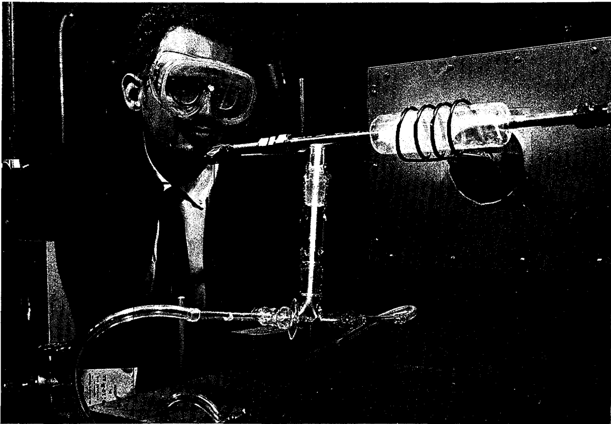
Fig. II-101. Plasma Magnetohydrodynamic Studies. Plasma conductivities must be measured to efficiently design magnetohydrodynamic nuclear reactor power systems. In the experiment shown here, the electrical conductivity of an uranium iodide-neon gas plasma (the lighted area within glass tubes) is being measured at Brookhaven National Laboratory. Other experiments have measured conductivities of plasma excited by metastable states of nitrogen. The measurements are made at relatively high pressures (several times that of normal atmosphere). Figure II-97 is another photo of the Brookhaven studies.
