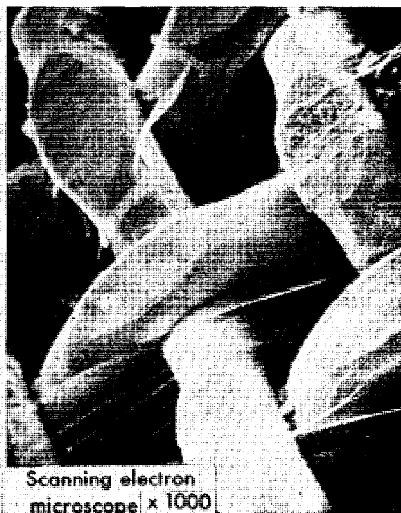
Figs. III-13 and 14. Scanning Electron Microscope. Photos above are a comparison of standard electron microscope (left) and scanning electron microscope (right) images showing how a stereoscopic view is possible with scanning electron microscope. Note that qualities such as the stainless steel 200-mesh woven grid being covered with a thin layer of plastic (Formuar) can be perceived with the scanning electron microscope. Schematic drawing on left shows basic scanning electron microscope system used in the new technique employed at Lawrence Radiation Laboratory, Berkeley, which can produce high-magnification, three-dimensional pictures.
