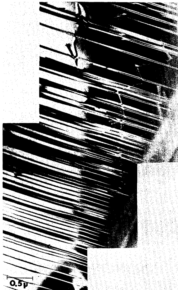
Figs. I-59 and 60. Dislocations in Ordered Alloys. Ames Laboratory micrograph on left shows nearly vertical dislocation pairs (double black lines) lying in the slip plane of the iron-silicon alloy that was oriented for single slip and deformed at room temperature. The scale at the left indicates 0.5 microns or 0.000020 inches. The dislocations are made visible since they represent a region of distortion in the crystal which interferes with and thus modifies the electron beam as it passes through these regions of the crystal in the electron microscope. On the right, a composite of several electron micrographs shows the nearly horizontal bands which are "mistakes" or antiphase boundaries produced by imperfect single dislocations generated during deformation at -30^{\circ} C. of a single crystal oriented for slip on only a single-slip plane. The section from which the picture shown above was taken, unlike the previous figure, was inclined 60^{\circ} to the slip plane. The antiphase boundaries being mistakes in the crystal are made visible by the electron beam from the electron microscope similar to the manner in which dislocations are made visible.
