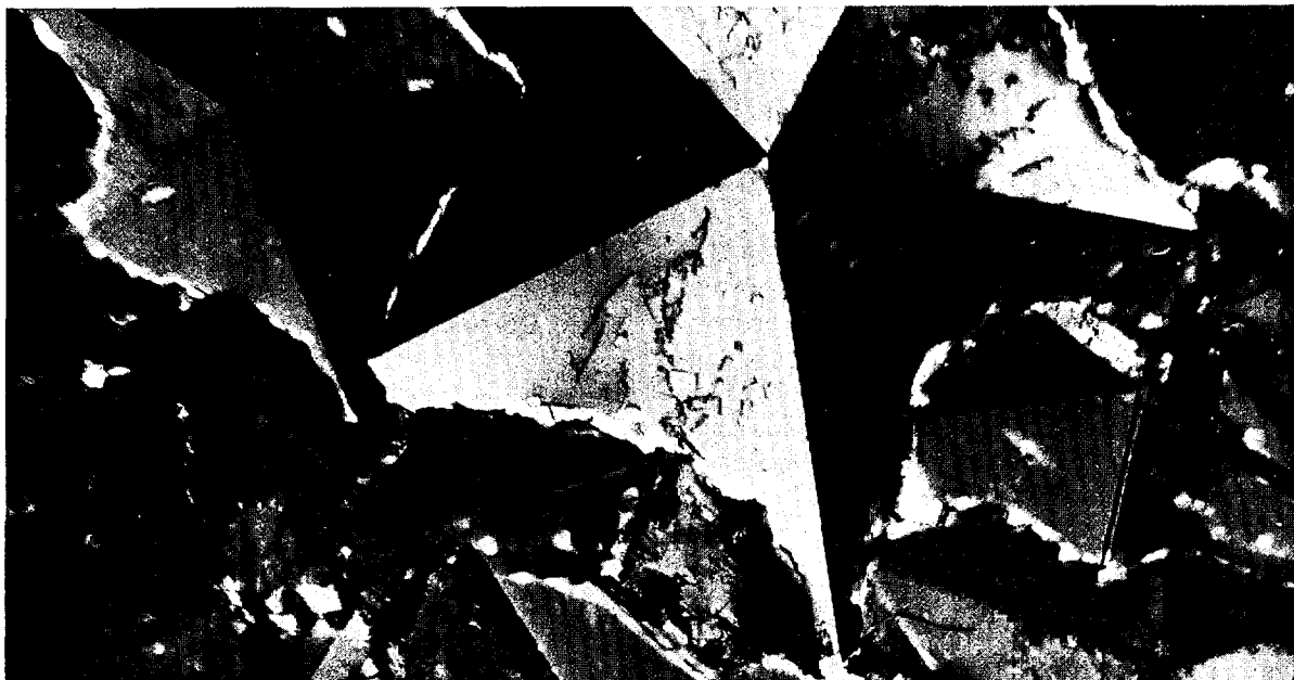
Figs. II-35 and 36. Pseudo-Fivefold Symmetry in Carbonyl Process Nickel. At Mound Laboratory, the effect of impurity gases on nickel coatings deposited by the thermal decomposition of nickel carbonyl [\text{Ni}(\text{CO})_4] is being studied. A transmission electron micrograph ( 40,000\times ) revealed grains which have apparent fivefold symmetry (shown above ). These are nearly perfect, fivefold twinned grains. The normal to the observed plane is the \langle 110 \rangle direction; the boundaries are parallel to (111) planes. The (111) planes of adjacent twin grains are separated by low-angle "tilt" boundaries. Five such boundaries account for five 1^\circ 28' mismatches. The angle between the (111) planes, which intersect along the \langle 110 \rangle direction, is 70^\circ 32' , instead of the 72^\circ needed for perfect fivefold twinning. Below is a transmission electron micrograph ( 50,000\times ) showing the general structure of a nickel coating made with a small quantity of hydrogen present in the carbonyl plating gas.
