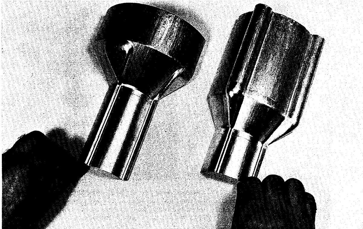
Figs. II-43 and 44. Cocxtrusion of Fuel Elements. Ribbed billets developed at Savannah River have eliminated the upset of the fuel core beneath ribs in extruded fuel tubes. The photo above shows a section of a composite tubular billet as it enters a die (broad portion) and a section of the ribbed fuel tube (small portion) that emerges. A round billet is shown on the left and a ribbed billet is shown on the right. The photo below shows a cross section of the rib area of a fuel tube. The core is a uranium-aluminum alloy, while the cladding is aluminum. The tube on the left was extruded from a round billet and shows the core upset. The tube on the right was extruded from a ribbed billet and has no upset. Reactor power can be increased by eliminating local temperature gradients, or fuel hot spots, caused by such core upsets.
