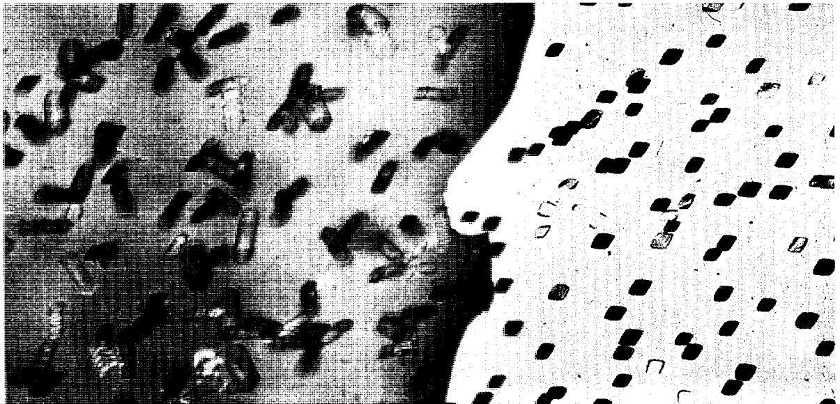
Figs. II-28 and 29. Fission Tracks. Photo above resulted from a Pacific Northwest Laboratory study of fission tracks and shows an irradiated sample of ordinary glass microscope slide coated with a thin layer of fissionable uranium. These tracks are actually trails of disrupted material caused by the passage of the fragments from the fissioning uranium. After irradiation, the glass was etched in hydrofluoric acid to enlarge the tracks for viewing in an optical microscope, as shown here with a magnification of 500\times . Photo below is of fission tracks in irradiated mica due to the fissioning of the natural-uranium impurities. This figure illustrates a technique developed at PNL to facilitate track counting. The right side of the figure shows the effect of coating a thin film of aluminum on the surface of the mica after etching. Tracks only on one surface are visible. The long track on the left side of the figure shows the full length of the track as it penetrates each layer of mica. The tracks are defined more clearly on the side coated with aluminum and, therefore, much easier to count.
