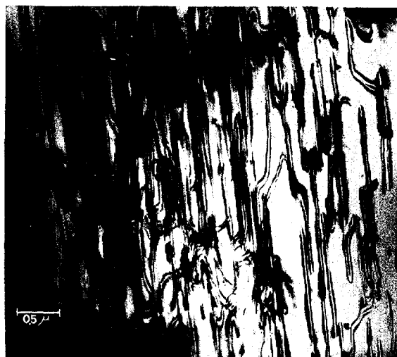
Figs. I-59 and 60. Dislocations in Ordered Alloys. Ames Laboratory micrograph on left shows nearly vertical dislocation pairs (double black lines) lying in the slip plane of the iron-silicon alloy that was oriented for single slip and deformed at room temperature. The scale at the left indicates 0.5 microns or 0.000020 inches. The dislocations are made visible since they represent a region of distortion in the crystal which interferes with and thus modifies the electron beam as it passes through these regions of the crystal in the electron microscope. On the right, a composite of several electron micrographs shows the nearly horizontal bands which are "mistakes" or antiphase boundaries produced by imperfect single dislocations generated during deformation at -30^{\circ} C. of a single crystal oriented for slip on only a single-slip plane. The section from which the picture shown above was taken, unlike the previous figure, was inclined 60^{\circ} to the slip plane. The antiphase boundaries being mistakes in the crystal are made visible by the electron beam from the electron microscope similar to the manner in which dislocations are made visible.
