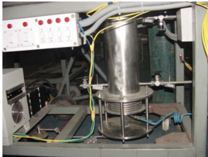
FIG. 6. Sodium bonding furnace housed below the glove box
