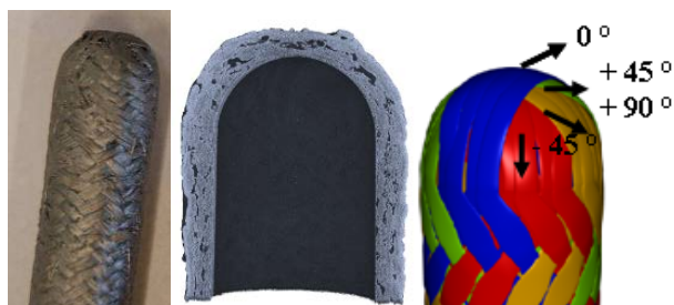
FIG. 4. CEA manufactured blind-end SiC/SiC-based cladding
