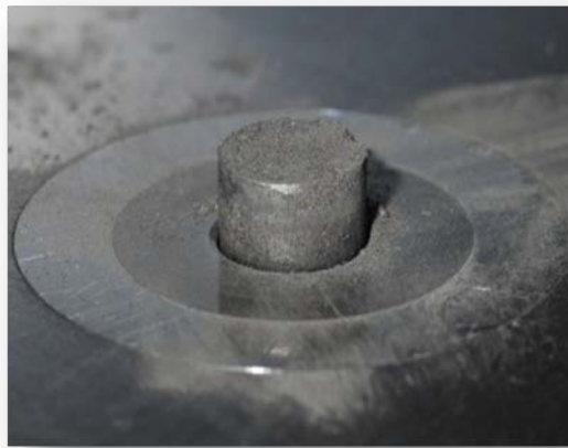
FIG. 9. Green compacts of metal uranium powder with the addition of 30 vol.% of chromium.
