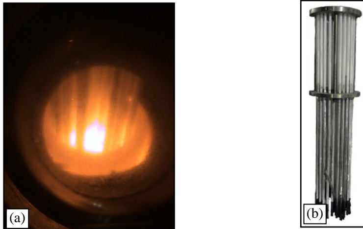
FIG. 4. Injection casting; (a) View of quartz tube moulds dipped in molten alloy, (b) Mould cassette holding cast slugs along with moulds
