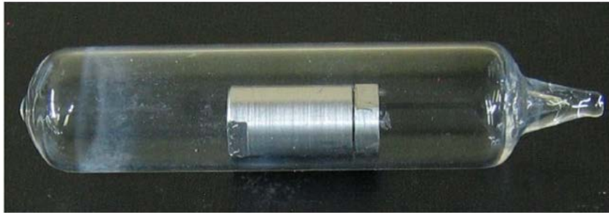
FIG. 2. Quartz encapsulated diffusion couple fixture.
