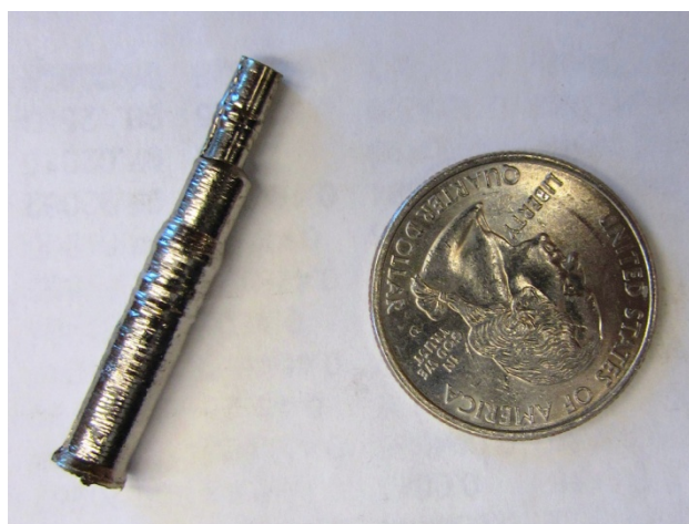
FIG. 1. A casting of a uranium alloy (a U.S. quarter, ~23 mm diameter, is placed in the figure for scale).
