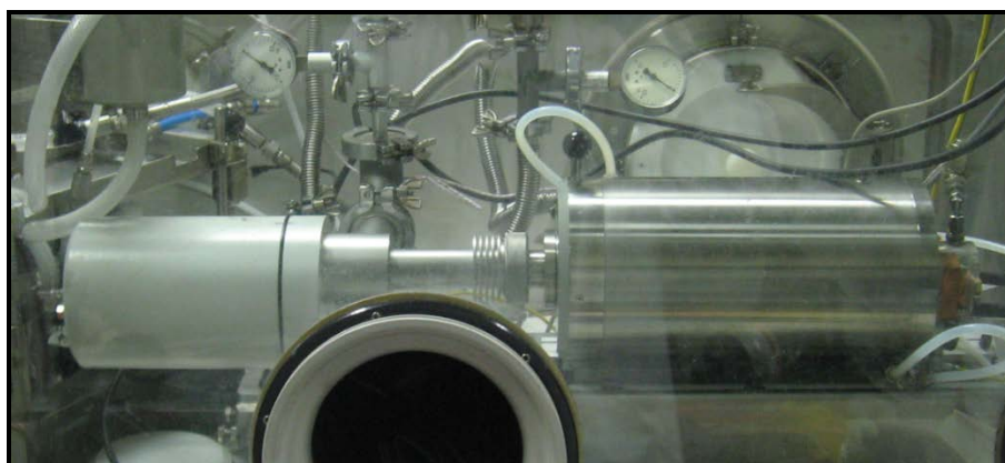
FIG. 2. Horizontal dilatometer integrated in glovebox at the CEA Marcoule Atalante facility.
