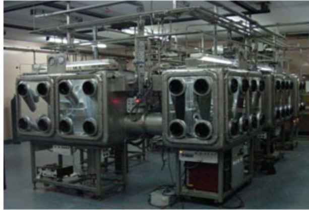
FIG. 2. Argon atmosphere negative pressure glove box train with various facilities
