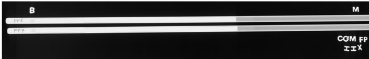
FIG. 7. X-radiography of the sodium bonded metallic test fuel pins
