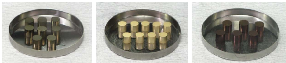
FIG. 1. From left, images of green ZrN pellets, sintered ZrN pellets and green (Zr_{0.6}Dy_{0.4})N pellets. A sintered (Zr_{0.6}Dy_{0.4})N pellet is nearly identical in its appearance to a sintered ZrN pellet
