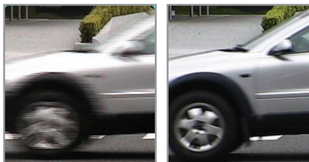
Progressive-scan CCD allows for the capture of clear, well-defined high-quality video of moving objects.
