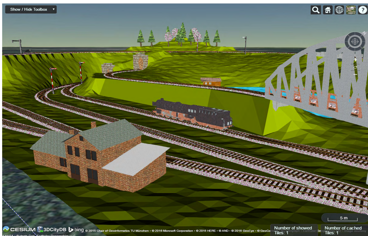
Figure 134: Screenshot showing the example of displaying different CityGML top-level features (building, bridge, tunnel, water, vegetation, transportation etc.) in glTF format in the 3D web client
