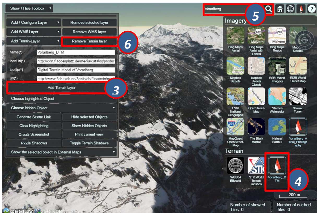
Figure 153: Example showing how to add a new terrain layer to the 3D web client
