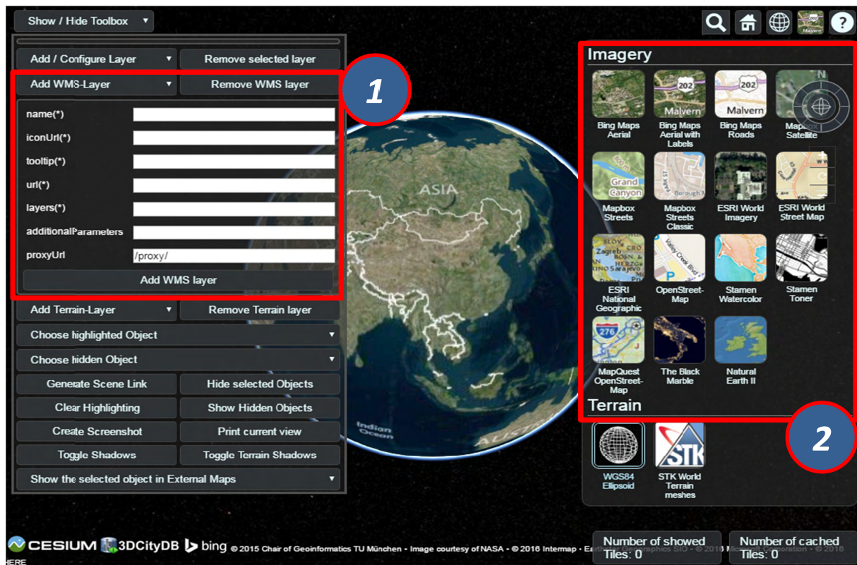
Figure 150: The input panel [1] for adding a new WMS layer and the BaseLayerPicker widget [2] where the added WMS layers will be listed together with the per default available imagery layers
