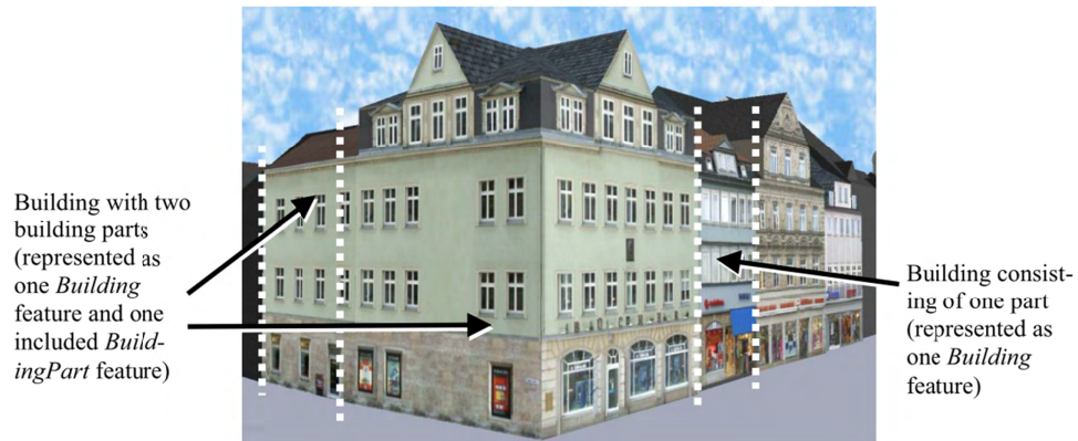
Figure 6: Example of buildings consisting of one and two building parts [Gröger et al., 2008]
