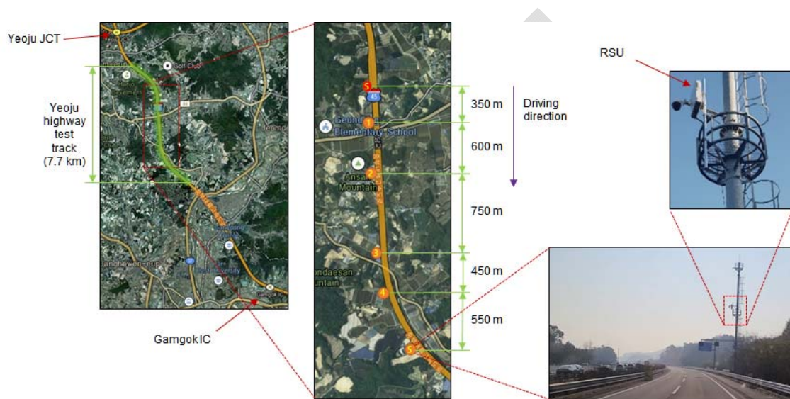
Figure 129: RSU deployment on a highway test track for Tethering via Vehicle scenario
