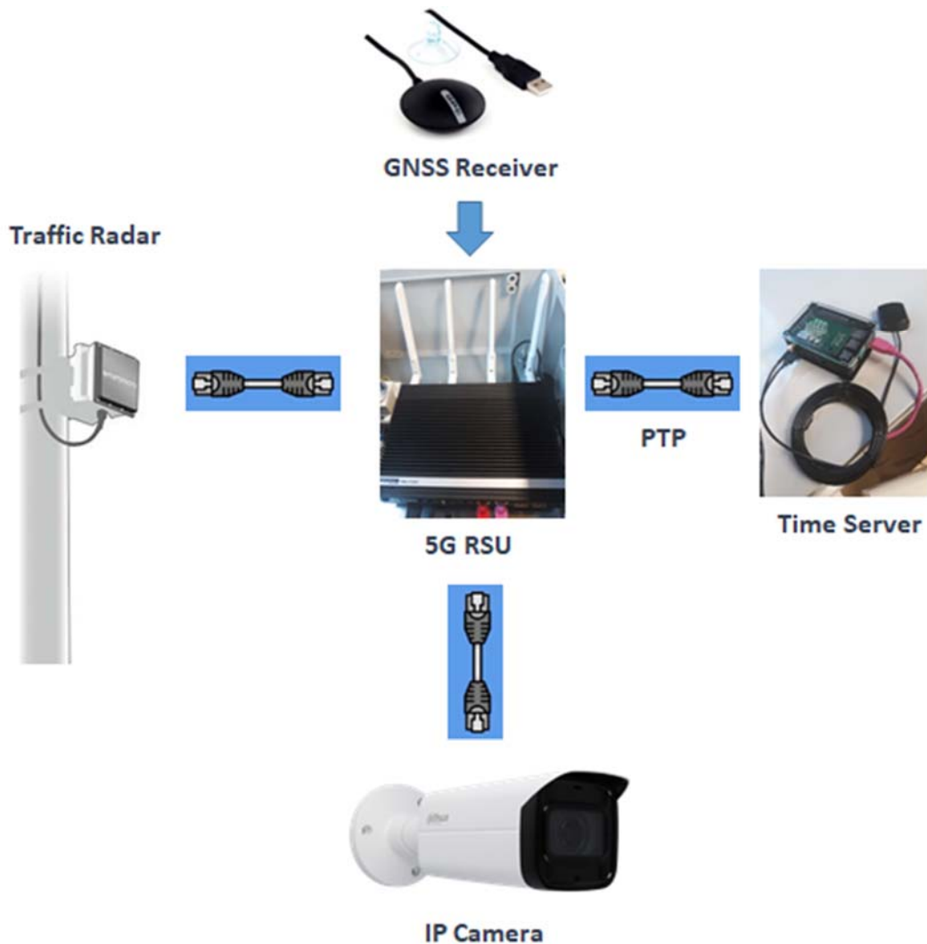
Figure 21: 5G RSU and roadside infrastructure equipment (PT side)
