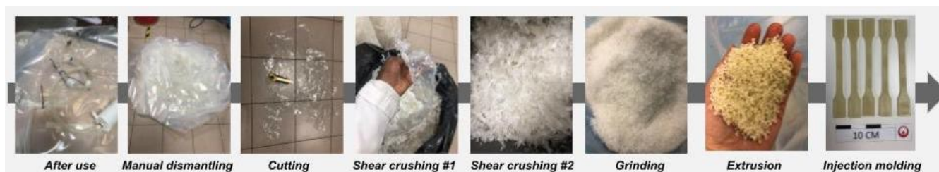
Fig. 3. Steps of material preparation of rLDPE_Pure.
