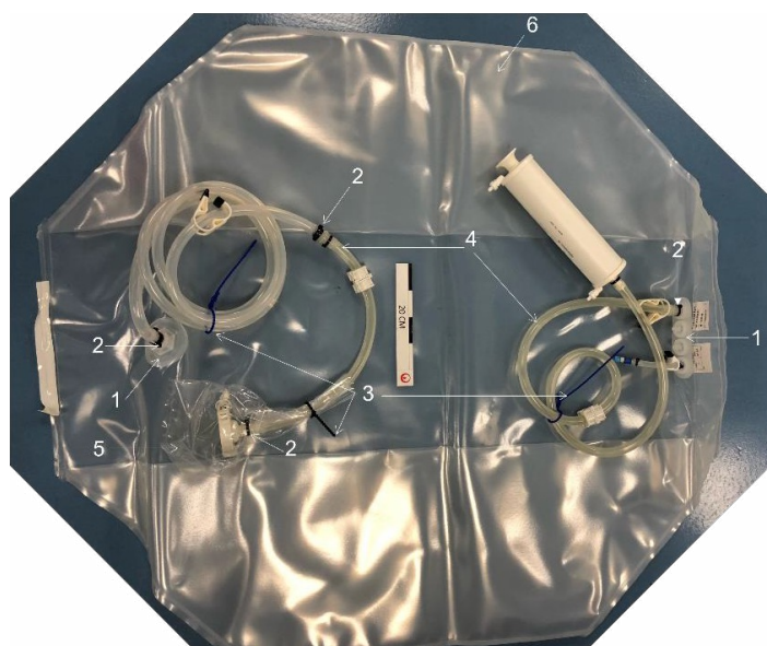
Fig. 2. Example of the structure of a bag: 1—cable tie, 2—bag port (welded on the film), 3—packaging tie, 4—tubes, 5—packaging overwrap, 6—film-bag chamber is composed of the film and the welded flange ports.
