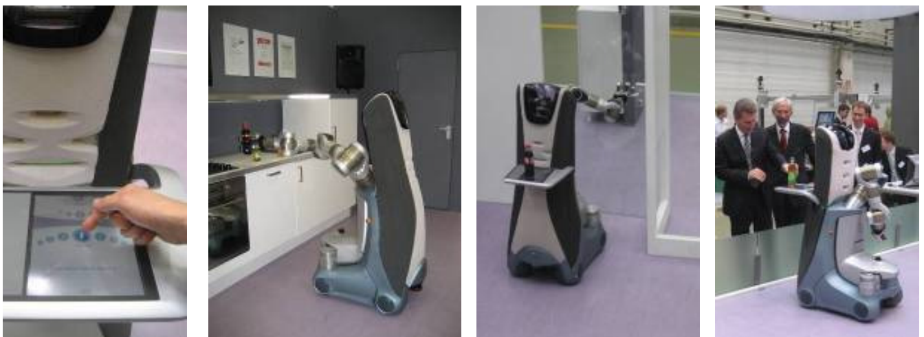
Fig. 8. Care-O-bot ® 3 executing fetch and carry tasks: order by touch screen, grasp a bottle, pass door, hand bottle and cup to visitors.
