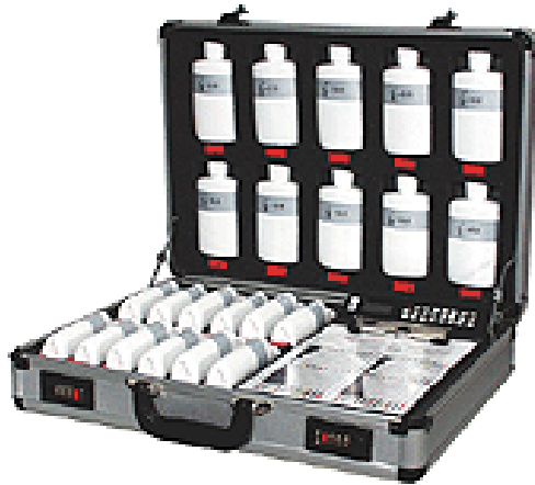
Figure 7. Two examples of modern detection threshold kits. Left: The Smell Threshold Test utilizing squeeze bottles to present different odorant concentrations of phenyl ethyl alcohol (rose oil) or amyl acetate (banana). Photo courtesy of Sensonics International, Haddon Heights, NJ USA. Right: Sniffin' Sticks. Phenyl ethyl alcohol or n-butanol odorants presented by felt-tip markers. Photo courtesy of Burghart Messtechnik GmbH, Wedel Germany.
