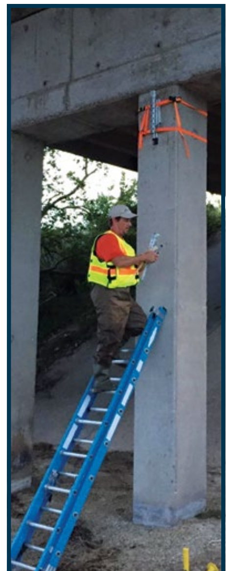
USGS scientist Charles Hartmann installs a storm-tide sensor in preparation for Hurricane Harvey in Carancahua Bay, Texas. Photo by George Umphres, USGS.
