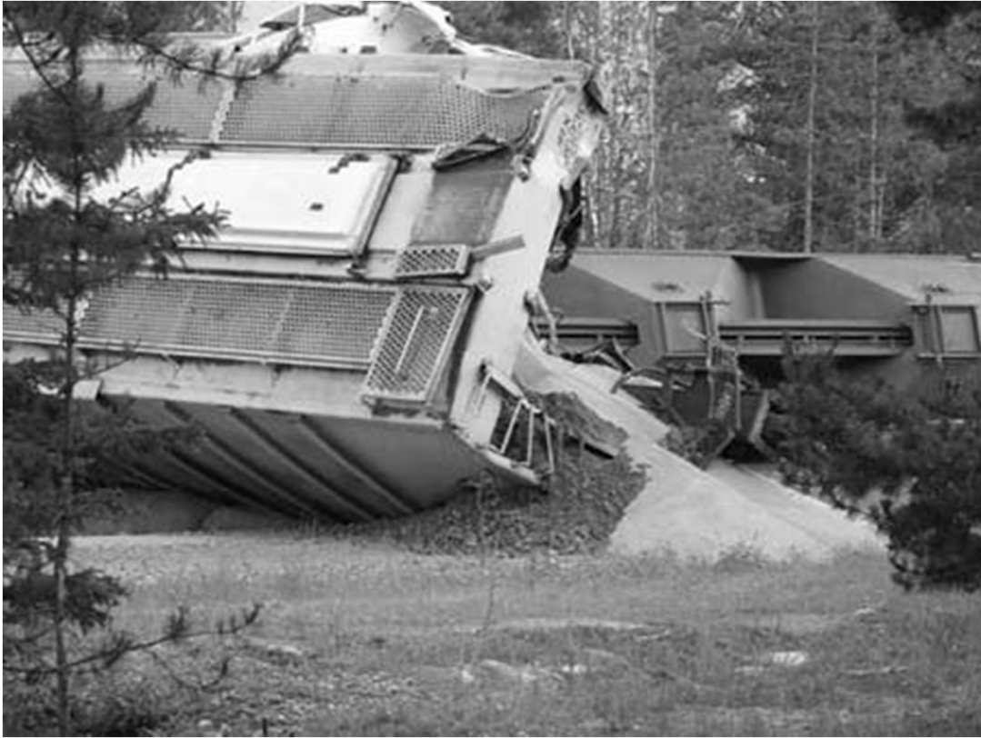
Plate 2. Photograph of a train derailment and grain spill in the Jasper townsite. “A CN Rail train lost a wheel and derailed near the town’s Petro Canada station June 29. A witness said the train was pulling out of the Jasper station when its wheel flew off, causing five cars to derail and grain to spill over the tracks, a pedestrian crossing and into the surrounding forest. Kolby Kongsrud submitted photo.” From Petersen (2008).
