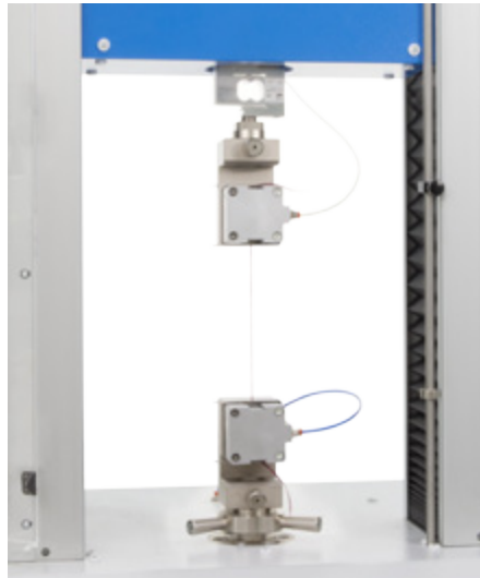
Pneumatic clamps for standard yarns and sewing threads up to 50N maximum resistance. Code 2510.982
