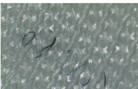
Defect analysis: presence of foreign coloured fibres in the fabric
