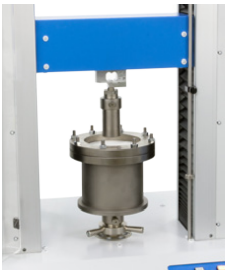
Tool for perforation test of non-wovens in compliance with UNI and ISO Standards (for Tensolab1000-5000 only) Type CBR. Code 2510.690
