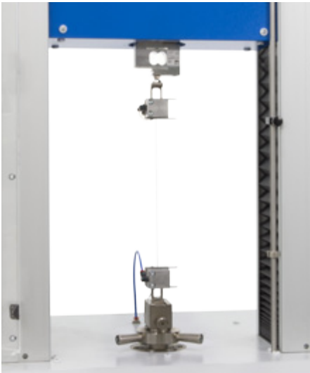
Pneumatic clamps for delicate yarns such as POY, Lycra, cotton and worsted yarns (20 N capacity). Code 2510.978
