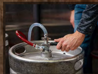
3.) Pull handle out and press downward until it locks into place. You are ready to draw beer
