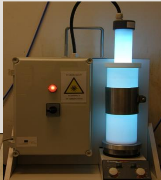
Annular batch photoreactor Oulu University Laboratory
