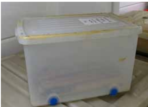
Plastic boxes such as this are good for short-term fixing of specimens - the plastic can become brittle and the lids usually don't have good seals, thus not good for long term storage
