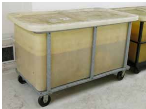
Large tanks such as this 1000L plastic tank with a wheel base are good for long-term storage and can be easily moved around.
