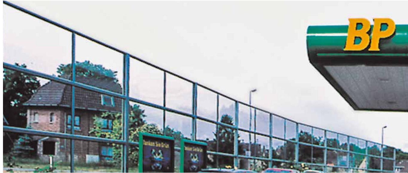
Noise barrier, gas station Wesseling PLEXIGLAS® Soundstop GS CC installed as an acrylic element with aluminum frame Alusyston Lärmschutz GmbH
