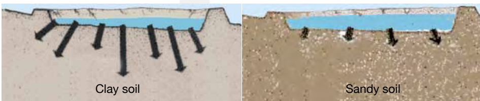
Figure 21. Waterproof qualities of clay and of sandy soil.
