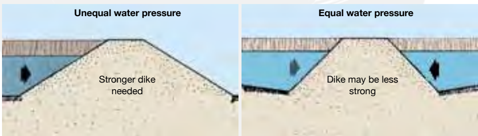
Figure 61. Dikes in different water pressure situations
