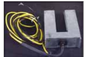
ARW470S1 Armor magnetic switch
