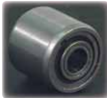
207BN1 Otis Ball Bearing, w/Double Row & Double Seal, O.D. 1.18", I.D. .39", 1.10"L
