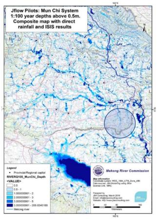
**Figure 13:** Map of projected flooding for the Mun Chi river basin (part of the LMB; the Young River Basin is highlighted by the circle).
