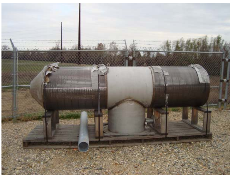
Photo 1 — Intake Structure with Wedgewire Screen Prior to Installation
