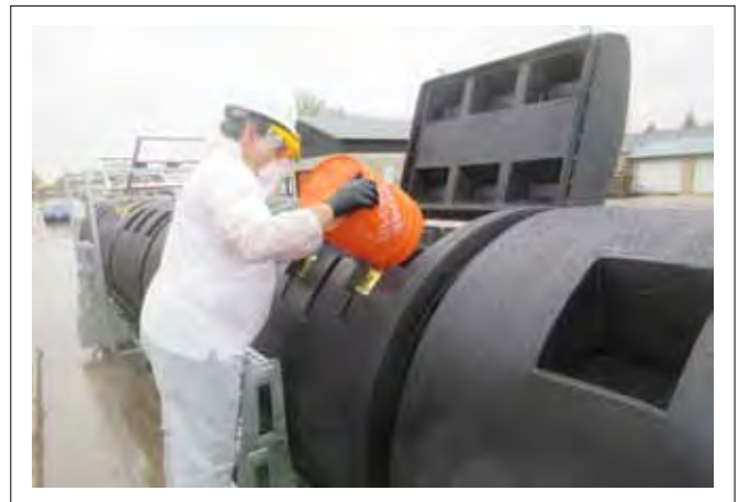
FIG. 5 ADDING BULKING (TYPICAL)
