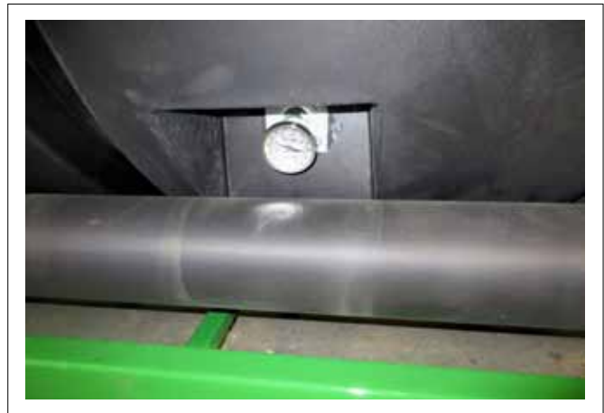
FIG. 49 TEMPERATURE GAUGES (TYPICAL)
