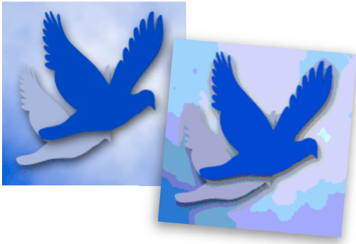
GIF image with selective color (left), and GIF image with web color (right)
