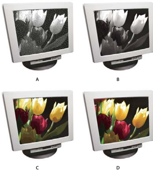
Image modes A. Bitmap mode B. Grayscale mode C. Indexed-color mode D. RGB mode
