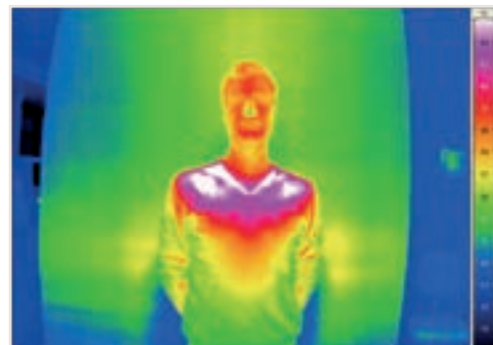
Heat spread at ambient temperature: 20°C, Spacing: ~ 2.0 m – After : After approx. 30 seconds IR short waves mainly heat objects, not the surrounding environment
