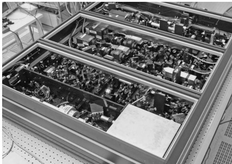
Fig.2: Photo of the GEO600 squeezed light source. More than one hundred optical components and various electronic control loops are required to prepare squeezed light for the application in a gravitational wave detector. Nevertheless, it is a compact construction with the dimensions of 135 cm x 113 cm at a total mass of about 130kg.
