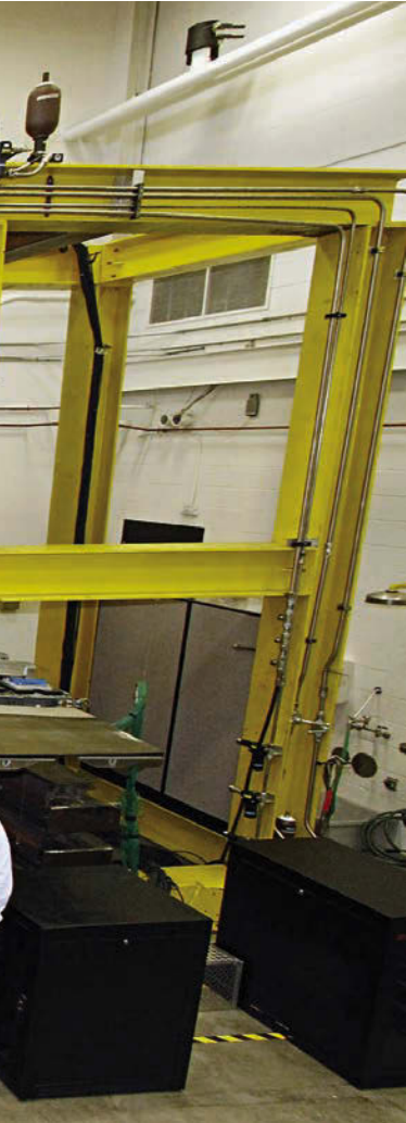
ABOVE: Applying C 3 Performance enabled NIAR to run this complex fatigue test of an F/A-18 Hornet composite wing structure 20% faster
