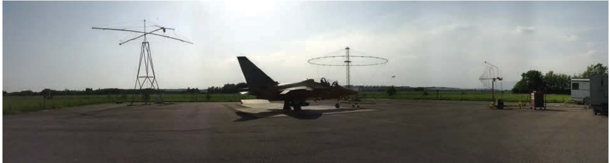
ABOVE: M346 outdoor electromagnetic test
