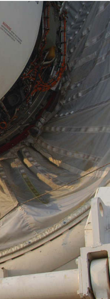
ABOVE AND LEFT: Arrays of microphones enable engineers to precisely identify near-field and far-field sound directivity
