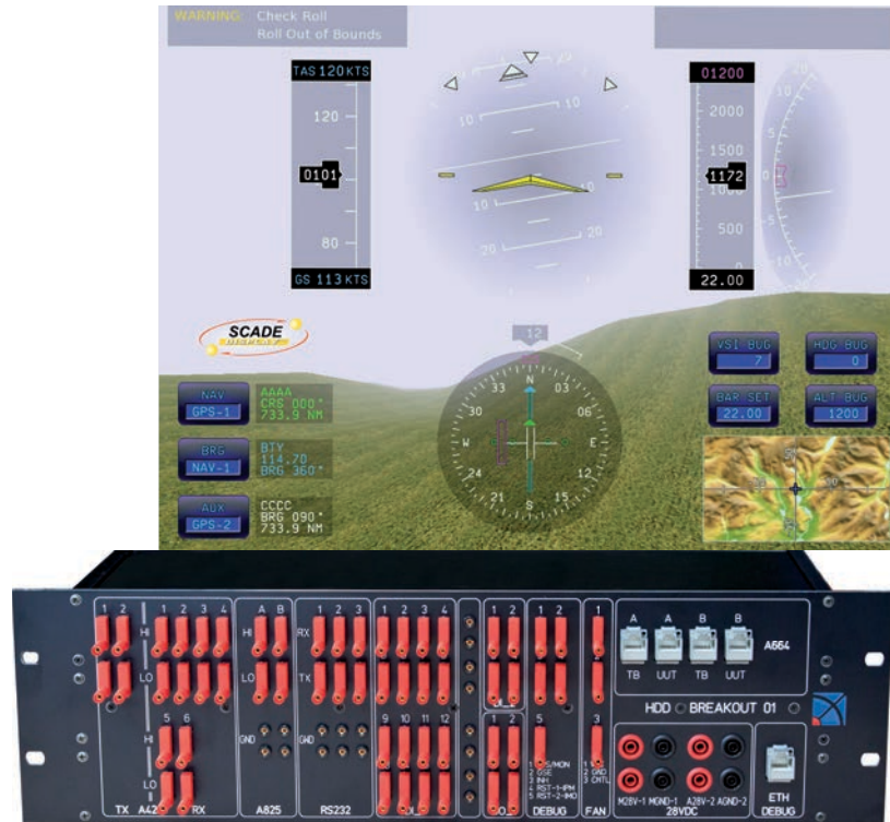
ABOVE: A customized SDIB breakout panel for a C919 multifunction display
