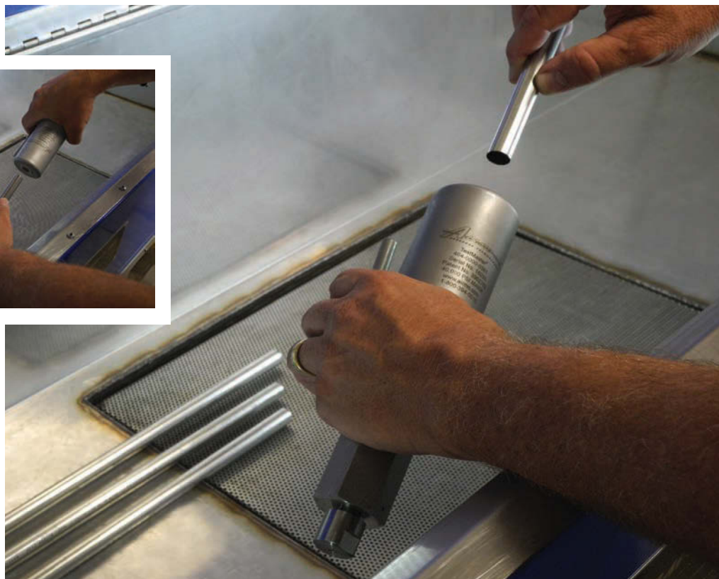
ABOVE: Inserting tube into fill side of hydrostatic test tool
