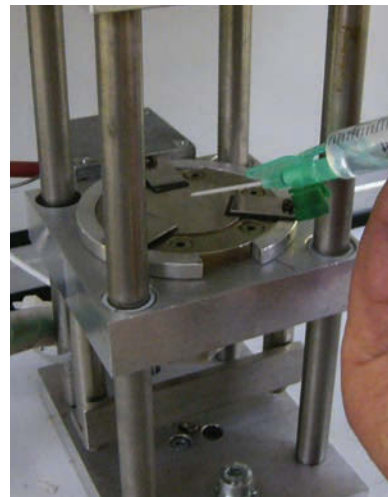
RIGHT, FIGURE 8: Small two-plate mold with integrated sensors
