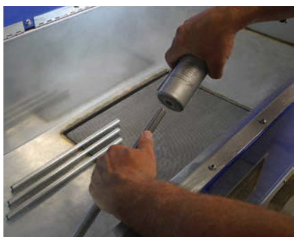
ABOVE: Inserting tube into fill side of hydrostatic test tool
