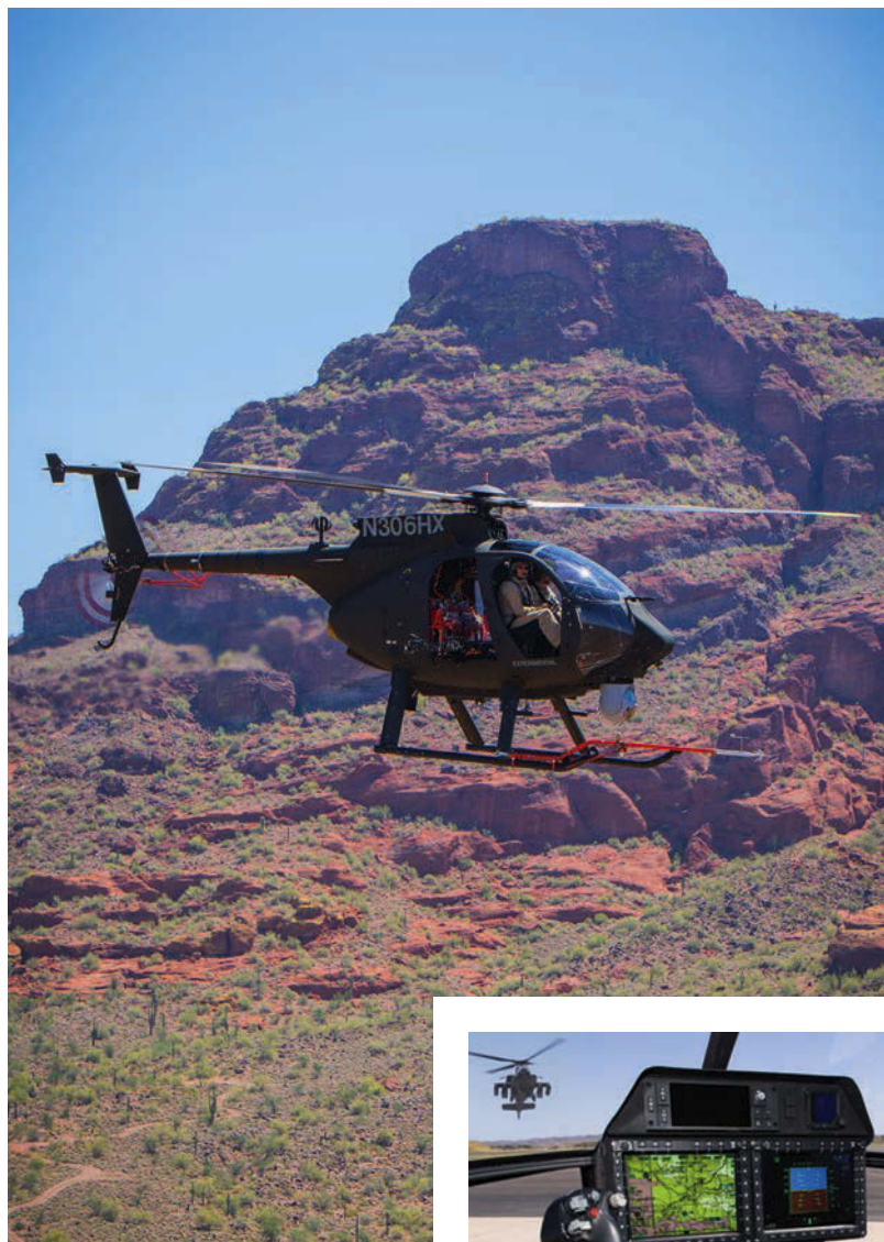
RIGHT: The production configuration AH-6i with 600hp drivetrain, six-bladed main rotor, canted tail rotor, and avionics 'beak' is under test for international customers
