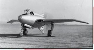
Sept. 6, 1943: Northrop's experimental fighter, the XP-56 Black Bullet was trucked to the Muroc lakebed and made its first flight, flown by company test pilot John Myers. The XP-56 was a near-tailless design with a pusher engine driving contra-rotating propellers. It was the first aircraft to be constructed entirely of magnesium.
