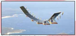
Sept. 8, 1999: The Helios Prototype flew for the first time at the Dryden (now Armstrong) Flight Research Center, Edwards, Calif. The Helios Prototype was the fourth and final aircraft developed as part of an evolutionary series of solar- and fuelcell-system-powered unmanned aerial vehicles. AeroVironment developed the vehicles under NASA's Environmental Research Aircraft and Sensor Technology program.
