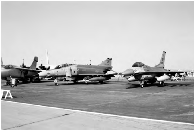
Two members of USAFE's EC Triad, the F-4G/F-16C Block 30D and the EF-111A. Both the F-4G and F-16C are configured with an AGM-88 HARM and ALQ-131. In addition, the F-16C carries AIM-9s and the F-4G an AGM-65 Maverick. The third member, the EC-130H, also flew combat sorties from Incirlik. (Tom Hanton)
