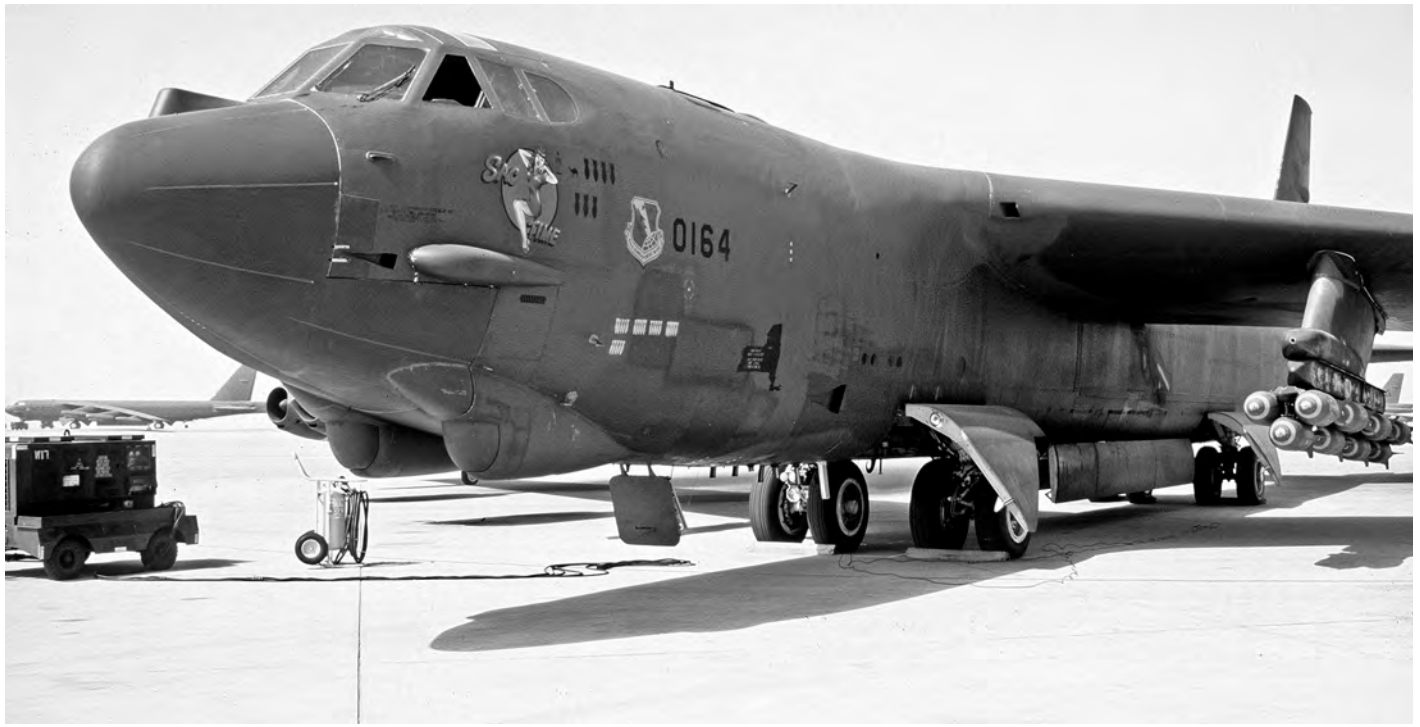
B-52G 58-0164 'SAC Time' of the 668th BS (416th BW, Griffiss) sits ready at Jeddah on February 1 for its next combat sortie. The BMWP 1708 aircraft is configured with M-117 750-pound bombs and already flew twenty-five combat sorties. (PH3 Chester Falkenhainer)
