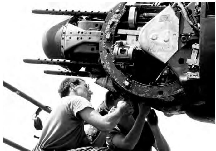
The B-52G still had its .50-caliber tail turret gun when it got involved in the Gulf War. However, the gunner had moved to the main crew compartment where he operated the gun by remote control. On the photo SSgt Brian Land checks the gun of a BMWP 1708 B-52G at Jeddah. (PH3 Chester Falkenhainer)
