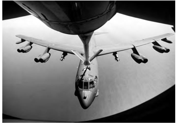
A B-52G is being refueled by a KC-135A while the BUFF is returning to its temporary base after flying a combat sortie. (USAF, SrA Chris Putnam)
