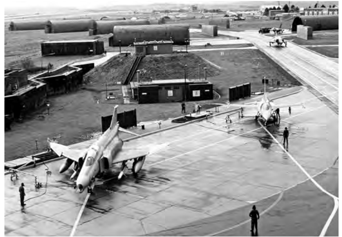
An F-4G and F-16C Block 30D on a wet Spangdahlem tarmac before deploying to Incirlik on January 17. The F-4G is configured with two AGM-88 HARMs and an ALQ-131 ECM pod, the F-16C carries two AIM-9 Sidewinders, two AIM-120 AMRAAMs and an ALQ-131. (USAF, 52nd TFW)
