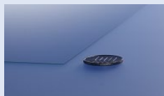
Comparison of 0.23 mm glass substrate for touchscreens with a coin
