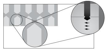
Fig. 4. The specimen is divided for the hardness test. Indentations are made in the upper surface of the specimen, before and after the unit is stored in ethanol.
