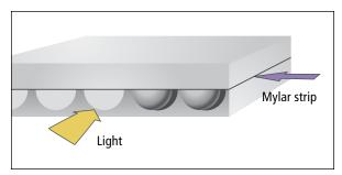
Fig. 3. A view of the insertion of composite, matrix position, and direction of light incidence during the polymerization process.
