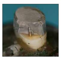
Fig. 9. A fracture within the amalgam at the pin/amalgam interface.
