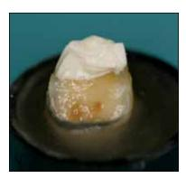
Fig. 12. A nonrestorable partial fracture within a specimen of CompCore AF without pins.
