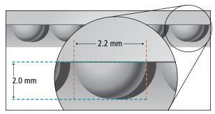
Fig. 1. A lateral view of the split mold, showing the 10 grooves and their lateral extension. The grooves are 2 mm high and 2.2 mm wide.
