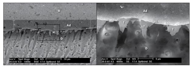
Fig. 2. *Left*: A micrograph of the adhesive interface from a specimen treated with the Optibond Solo Plus SE system and restored with Point 4 composite resin (magnification 1,000x). *Right*: A micrograph of the central portion of this specimen (magnification 4,000x) reveals the anatomy of the extremely irregular, short tags. Ad = adhesive; HL = hybrid layer; D = dentin; R = resin; T = tag.
