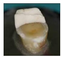
Fig. 10. A partial fracture within a CompCore AF specimen without pins.
