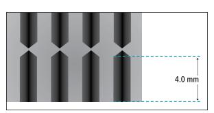
Fig. 2. An upper view of the inferior part of the mold and the length of the grooves (4 mm), which simulates the depth.
