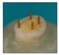
Fig. 2. A specimen with four TMS Link Plus Regular pins.
