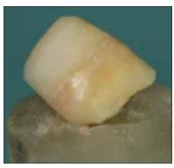
Fig. 7. Root fracture of a FluoroCore 2 specimen retained by pins and Optibond Solo Plus with BondLink. The core foundation remained intact.
