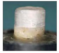
Fig. 5. A Tytin specimen with a 1 mm bevel at the axial-occlusal line angle.
