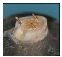
Fig. 13. A specimen of CompCore AF, with pins bending away from the applied force.
