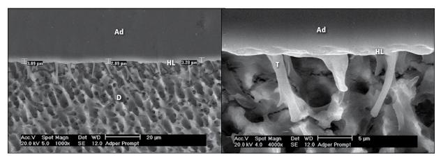
Fig. 3. *Left*: A micrograph of the adhesive interface of occlusal dentin from a specimen treated with the Adper Prompt adhesive system and restored with Filtek Z250 composite resin in a dentin slice of the occlusal surface (magnification 1,000x). The dentinal tubules can be seen perpendicular to the restoration. *Right*: The central area of the sample (magnification 4,000x) indicates short, irregular tags can be observed. HL = hybrid layer; T = tag; Ad = adhesive; D = dentin.
