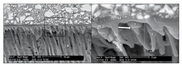
Fig. 1. *Left*: A micrograph of the adhesive interface from a slice of occlusal dentin treated with the Clearfil SE Bond adhesive system and restored with Clearfil APX composite resin (magnification 1,000x). *Right*: A micrograph of the central portion of this specimen (magnification 4,000x). Ad = adhesive; HL = hybrid layer; D = dentin; R = resin; T = taq.
