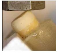
Fig. 6. A FluoroCore 2 specimen in the universal testing machine.
