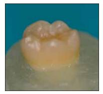
Fig. 1. A specimen mounted in acrylic resin.
