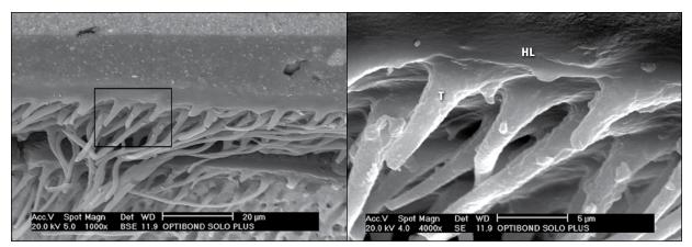
Fig. 5. *Left*: A micrograph of the adhesive interface of occlusal dentin from a specimen treated with the Optibond Solo Plus adhesive system and restored with Point 4 composite resin (magnification 1,000x). *Right*: The central area of this specimen (magnification 4,000x). HL = hybrid layer; T = tag.
