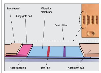
Fig. 1. The lateral flow immunochromatography platform.
