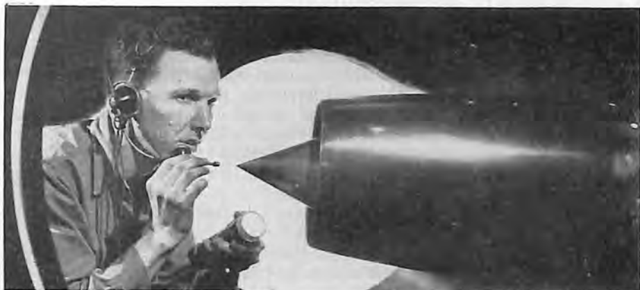
NACA engineer checks supersonic ramjet engine for test
