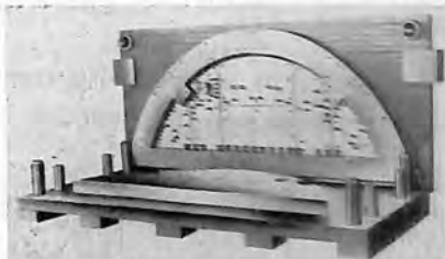
TWIX made Compound Blank and Pierce Die. 136 No. 40 holes and Perimeter; 60" long x 30" wide.
