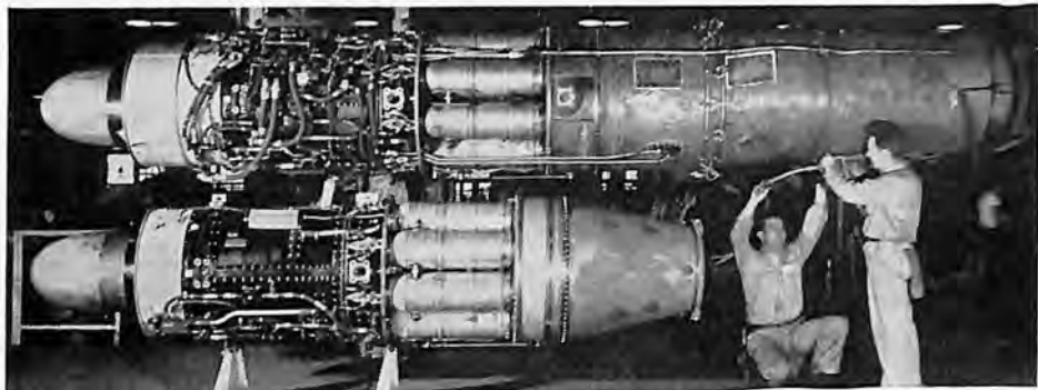
General Electric J47-GE-17 with afterburner and standard J47-GE-11 model below
