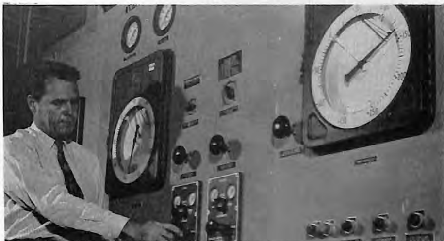
Engineer adjusts main control panel of Northrop fuel system test laboratory to check simulated altitude performance
