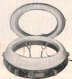
Routing and Drill Fixture made of Ren-ite
