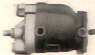
The 66W Series of STRATOPOWER Hydraulic Pumps embrace a range of models from 2 to 10 gpm at 1500 rpm with continuous pressures to 3000 psi. Designed for maximum continuous speed of 3750 rpm . . . intermittent speeds to 4500 rpm.
