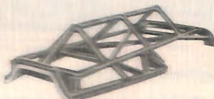
Canopy Opening Checking Fixture, showing the use of Ren-ite Plastic stock tubing
