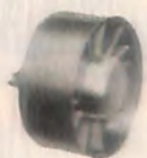
Ram air turbine driven unit for emergency aircraft power.
