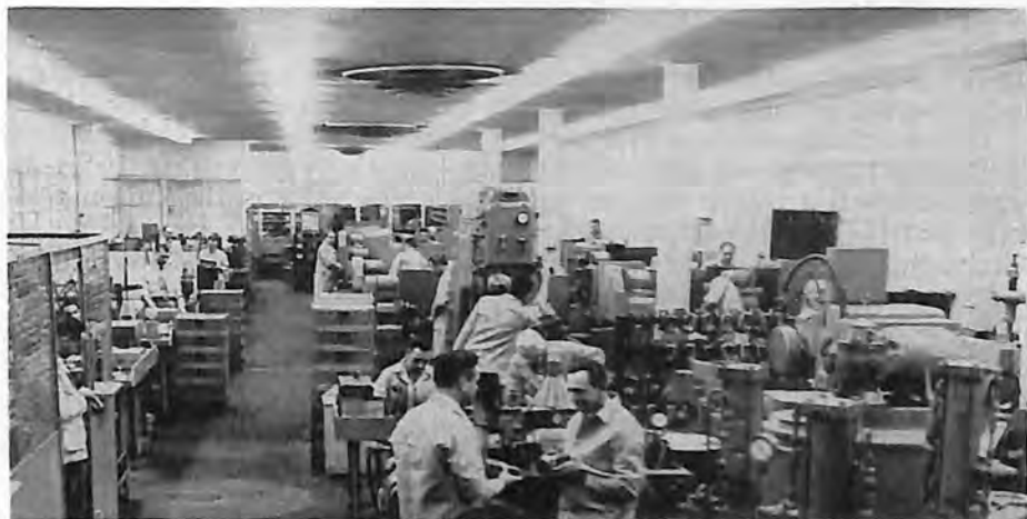
Gyro parts are machined in glass-enclosed, temperature and humidity-controlled laboratory room at Bendix Eclipse-Pioneer Division
