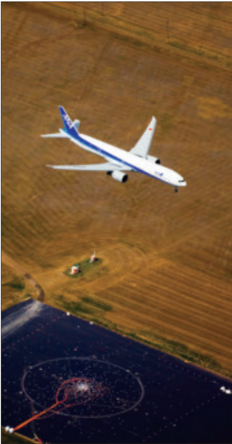
A flyover noise test of Boeing's 787 aircraft used a ground array consisting of 614 microphones.
