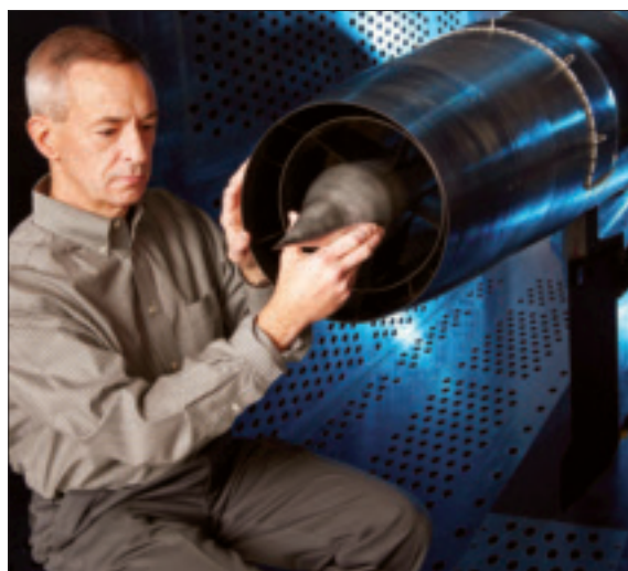
NASA engineer Rod Chima works with a low-boom 'relaxed-compression' inlet installed for testing in the NASA Glenn 8x6-ft Supersonic Wind Tunnel.
