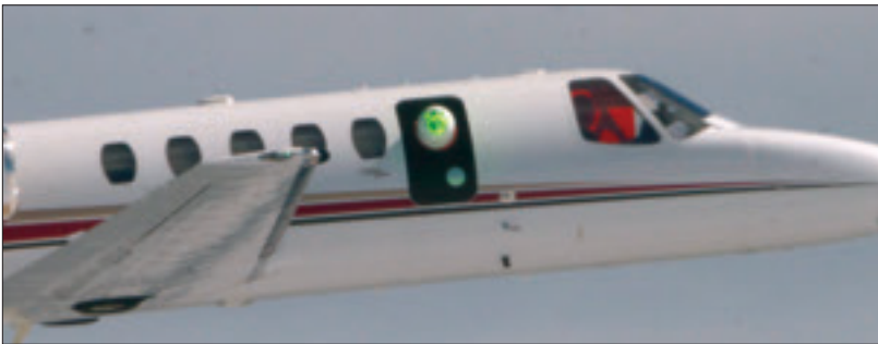
The laser turret and testing configuration for the Airborne Aero-Optics Laboratory at the University of Notre Dame are carried aloft.
