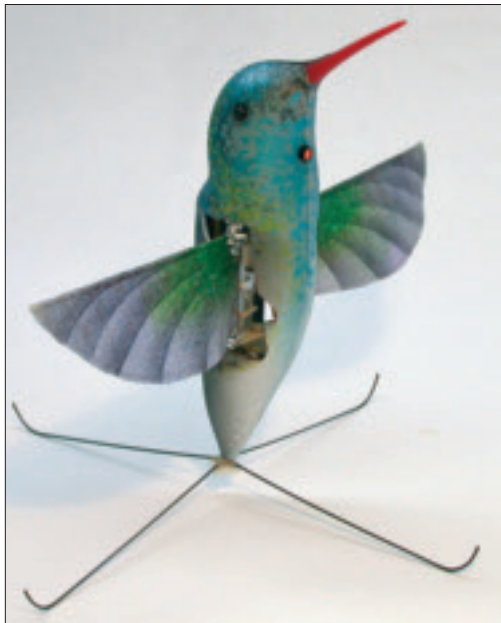
The Nano Hummingbird can fly for up to 10 min, streaming video back to a base station.
