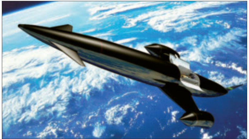
Skylon's SABRE engines use liquid hydrogen combined with oxygen from the air at altitudes of 26 km and speeds of up to Mach 5. Credit: Reaction Engines.
