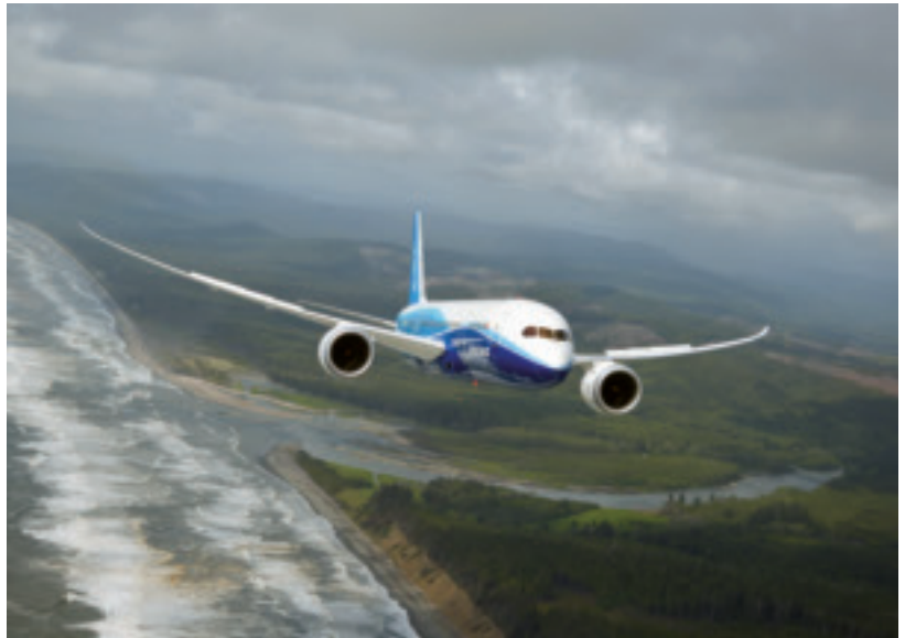
Flight control software on the 787 allows for optimizing wing camber in flight.
