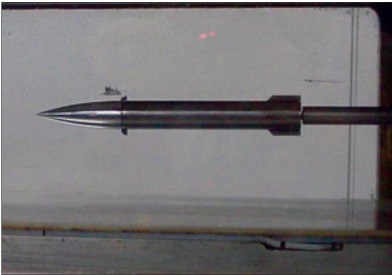
A steerable adaptive bullet awaits Mach 3 testing in a supersonic wind tunnel.
