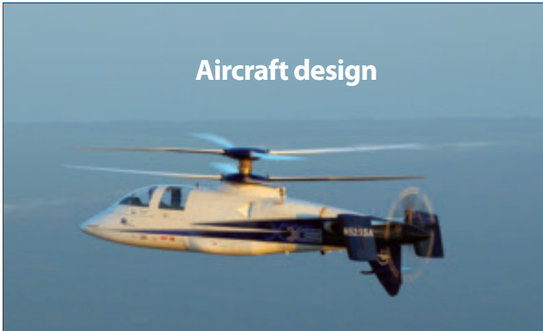
The X2 technology demonstrator sets a 250-kt cruise speed record, using its tail-mounted pusher prop. The helicopter's contra-rotating coaxial rotors slow as it accelerates.
