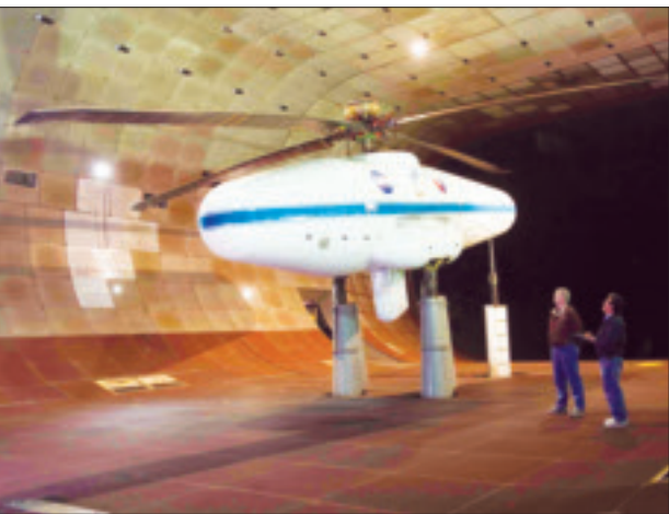
NASA and the Army have begun detailed analysis and correlation efforts with data acquired during the 2010 UH-60A airloads wind tunnel test.
