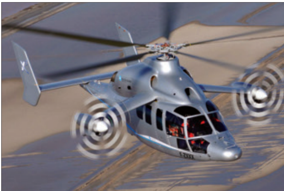
Eurocopter's X3 hybrid helicopter achieved an airspeed of 232 kt on May 12.
