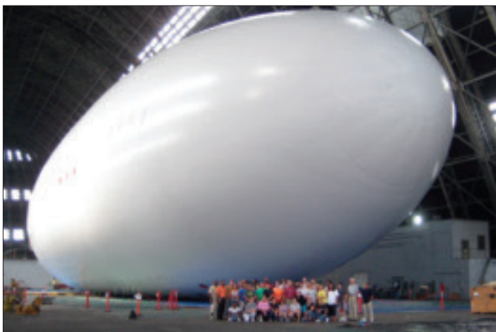
The envelope of the Blue Devil airship is inflated with air.
