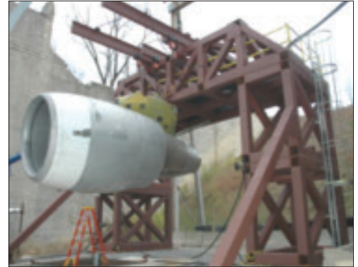
A large turbofan engine mounted on a test stand awaits MANPADS testing.
