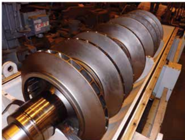
▲ Figure 10. Electroless nickel coatings are more durable than PTFE coatings, and can remain intact for many years. The coating shown here has been in operation for six years. Photo courtesy of Elliot Group.
