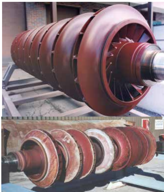
▲ Figure 9. PTFE coatings offer good corrosion resistance in many applications, but are not very durable. This coating is shown brand new (top) and after 18 months in service (bottom). Photos courtesy of Elliot Group.
