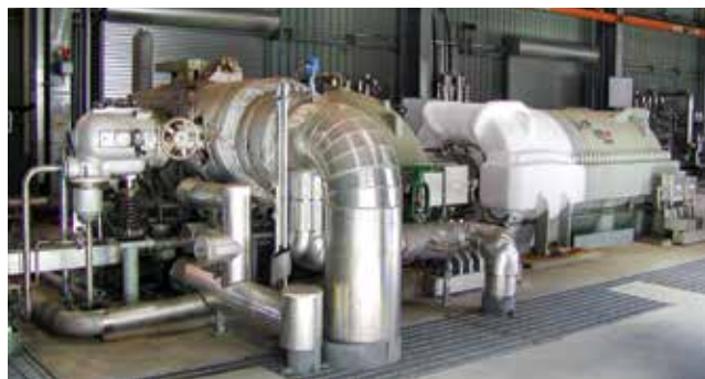
▲ Figure 5. Centrifugal compressors in ethylene plants come in varying configurations and can handle large volumes. Photo courtesy of Elliot Group.
