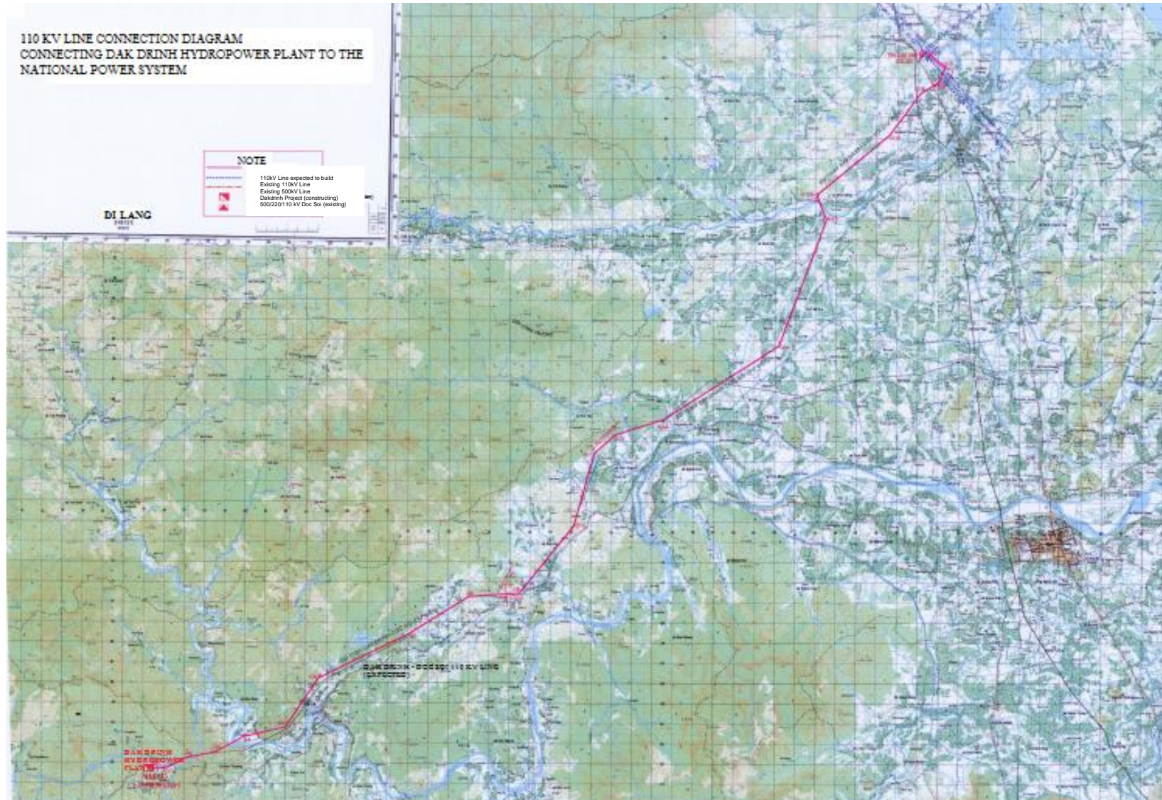
Figure 1.4: ROUTE DIAGRAM OF THE 110 KV LINE CONNECTING DAK DRINH HYDROPOWER PLANT TO NATIONAL POWER SYSTEM
